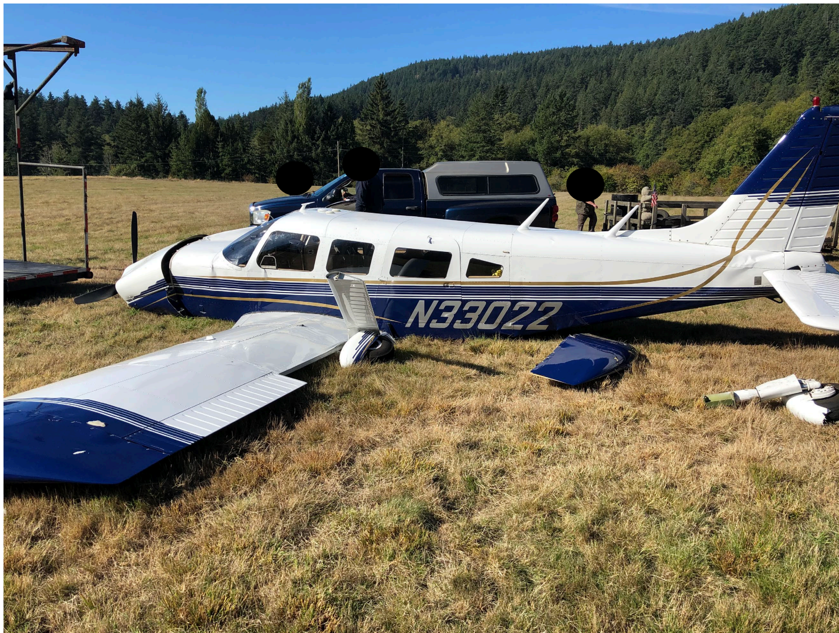
Photo 1 – View of airplane in open field with damage to left wing and fuselage (courtesy of recovery company)
