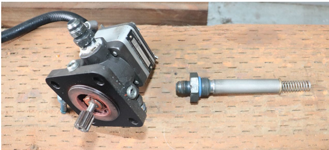
Figure 6. A picture of the fuel pump and fuel flow servo fuel filter
