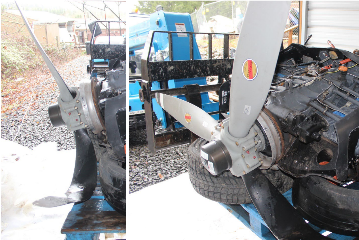
Figure 8. Two viewpoint pictures of propeller blades and hub assembly
