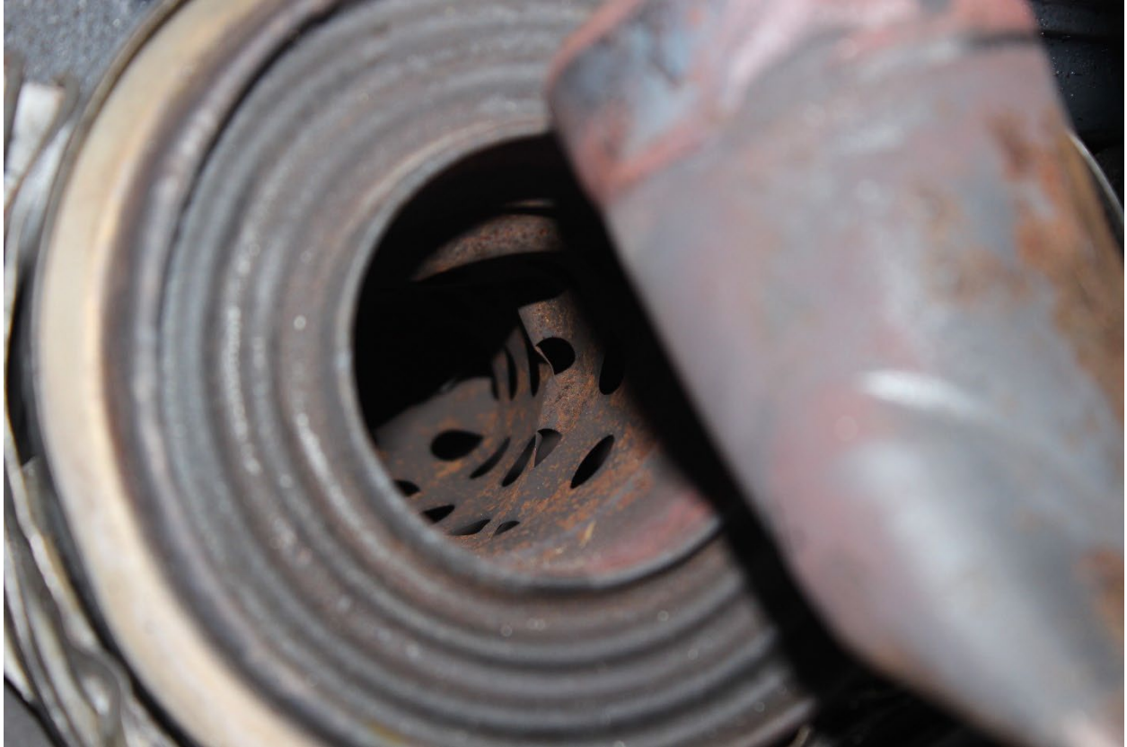
Figure 7. A picture of muffler and its internal metal lining.
