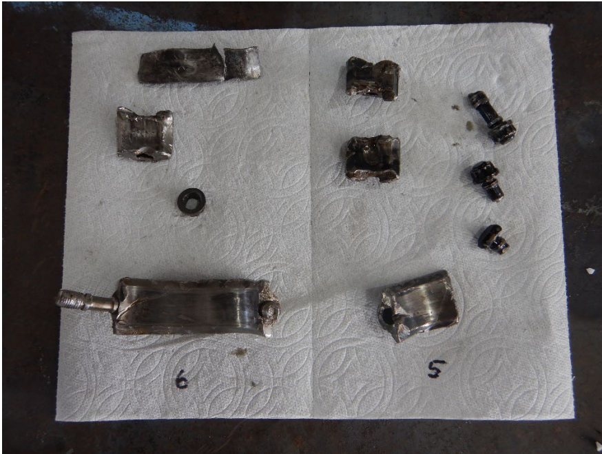
Photo 6 - View of Connecting Rod Pieces and Hardware
