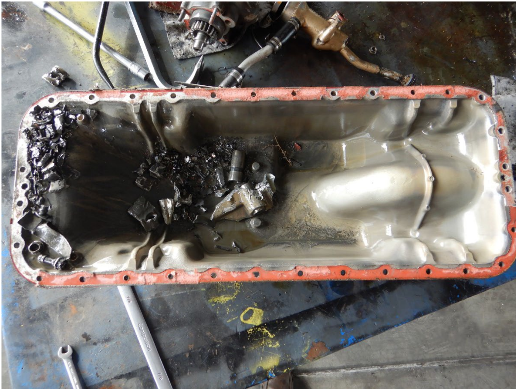
Photo 5 - View of Oil Sump
