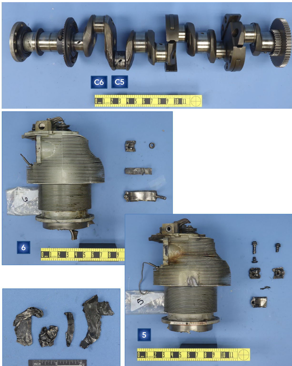
Figure 1. Overall views of the submitted crankshaft (upper image), number 5 cylinder and associated connecting rod pieces, and bearing pieces (lower images), and number 6 cylinder with connecting rod pieces and a bearing half (middle image).
