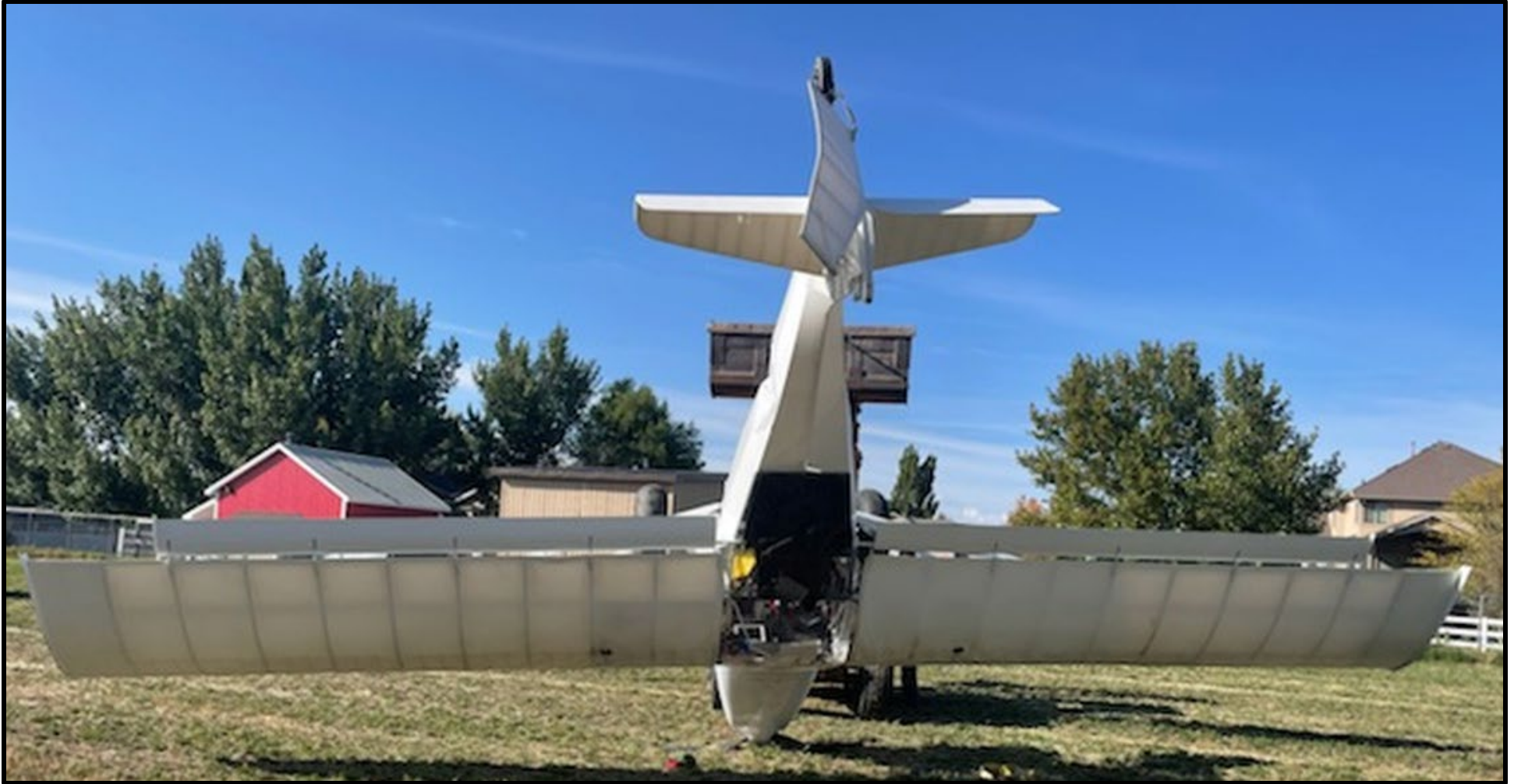
Figure 2: Airplane Being Recovered Showing Damage of Rudder (photo provided by Weber County Sherriff)
