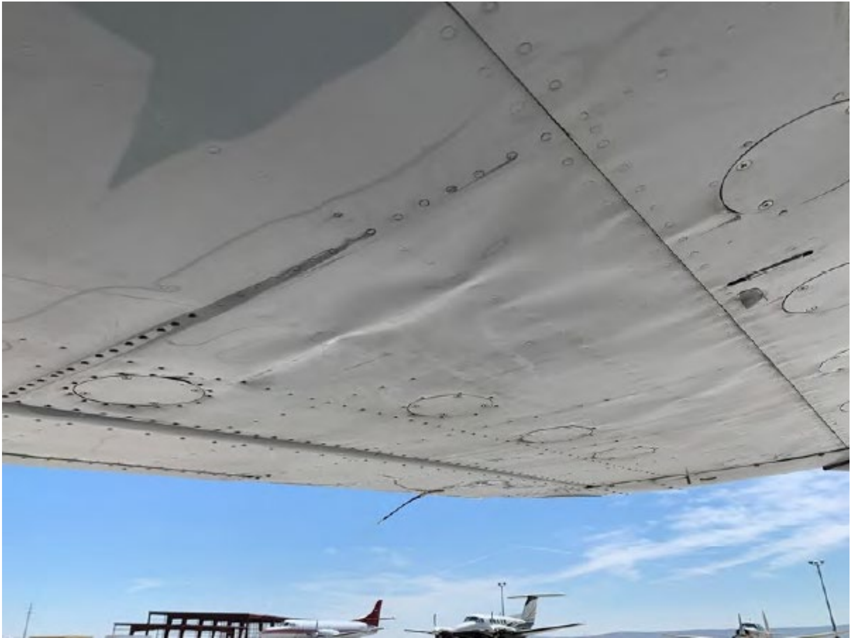
Photo 1 – View of damage to the right wing (courtesy of the Insurance Adjuster)
