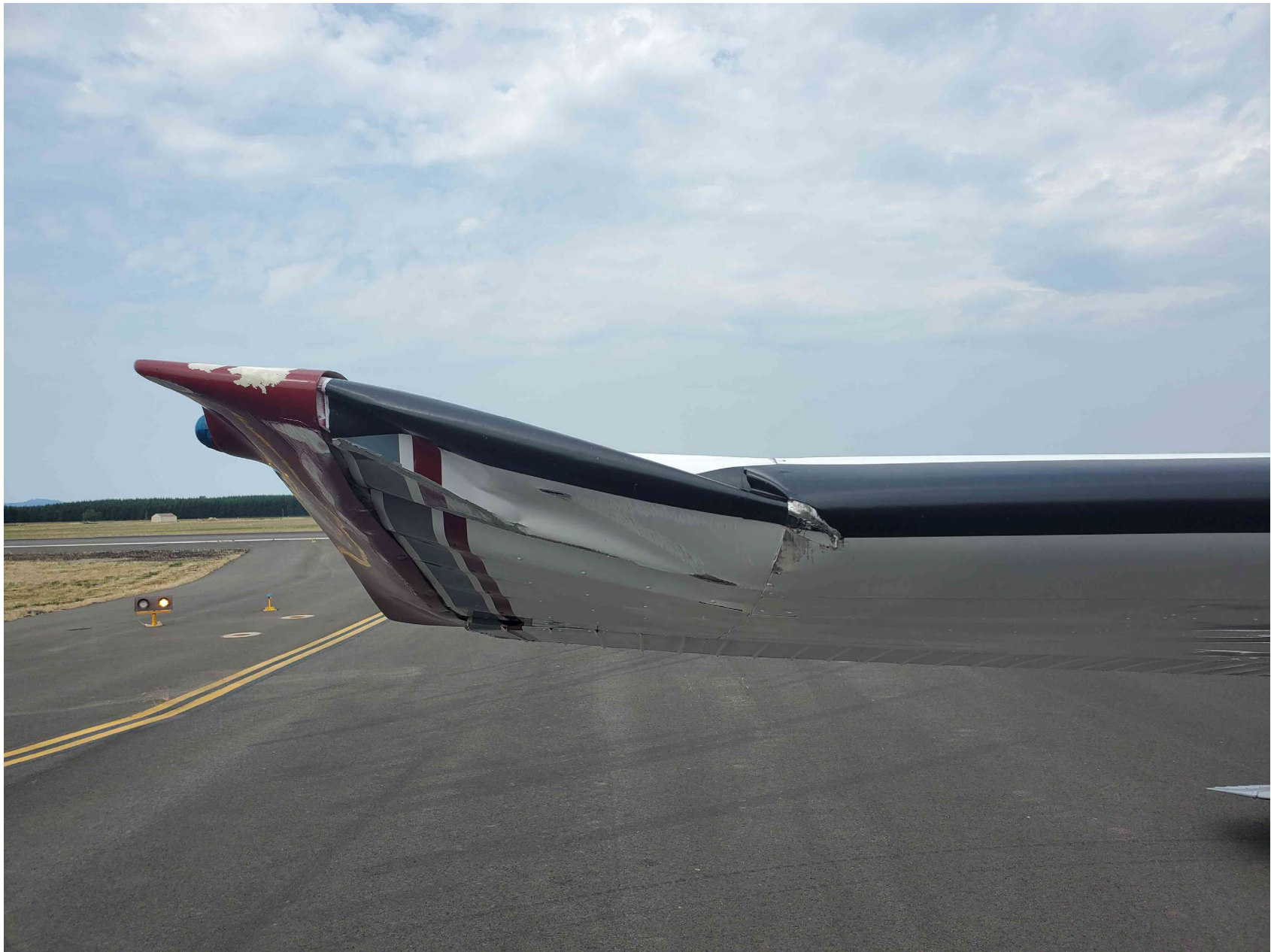
Photo 2 – Right wing damage
