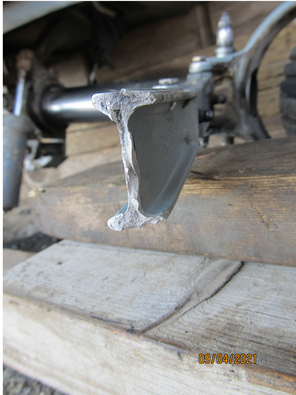
Photo 2 – Lower section of the nose gear upper torque link. Photo courtesy of the pilot.
