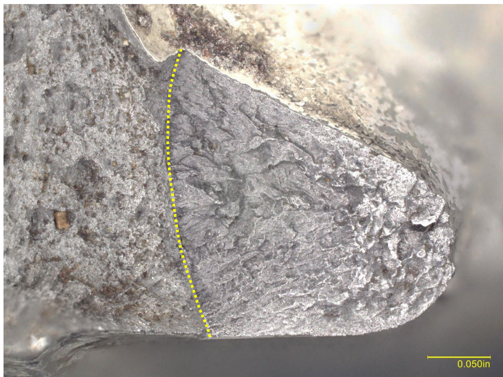
Figure 6. Digital microscope images showing the flat area (yellow bracket) on the fracture surface of the bottom rib indicated in Figure 4. The yellow dotted line delineates the edge of the flat area.
