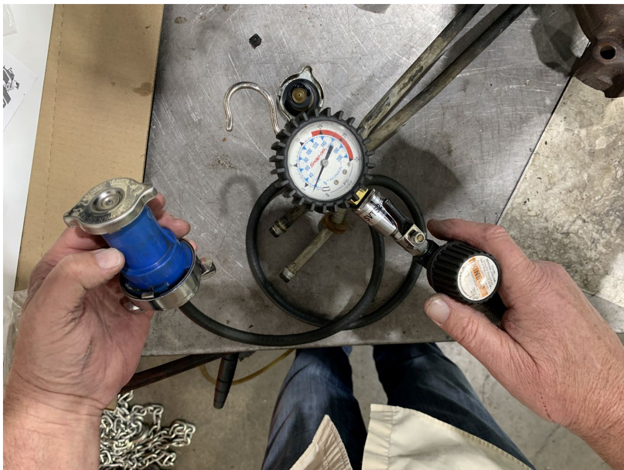
Figure 9. View of radiator cap return valve test result
