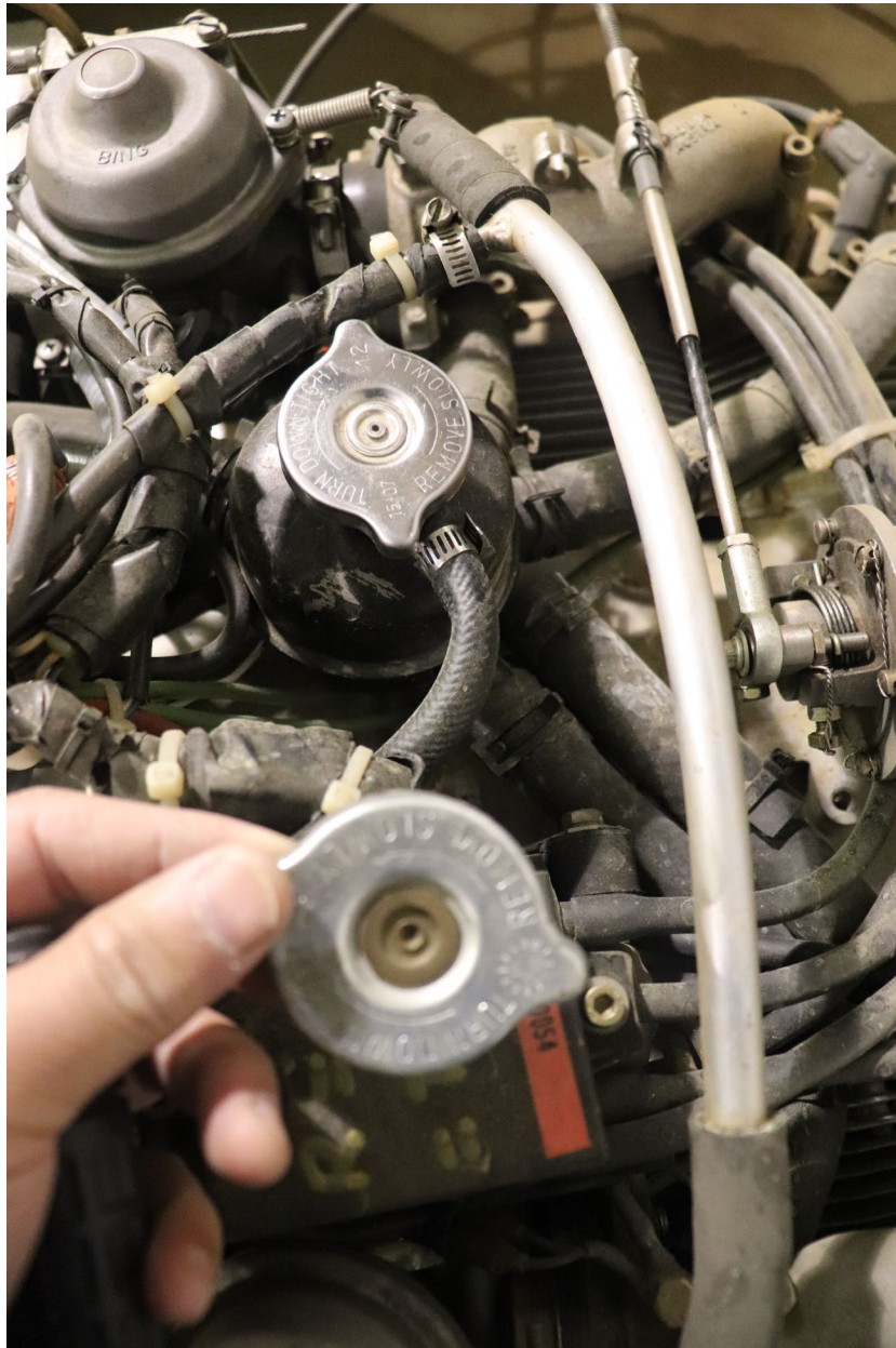
Figure 7. View of non-OEM installed on expansion tank comparing with the removed Rotax radiator cap
