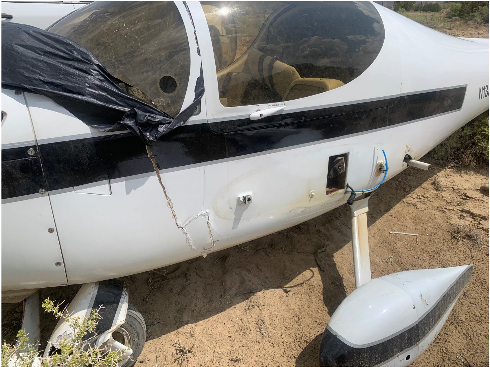
Photo 2 – View of left side damage to fuselage (courtesy of the pilot)
