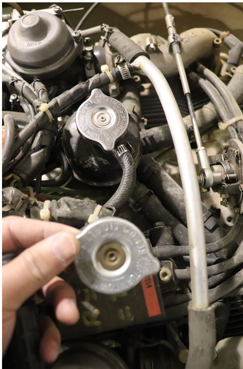
Photo 6 – View of installed non-Rotax radiator cap installed on expansion tank and original Rotax radiator cap
