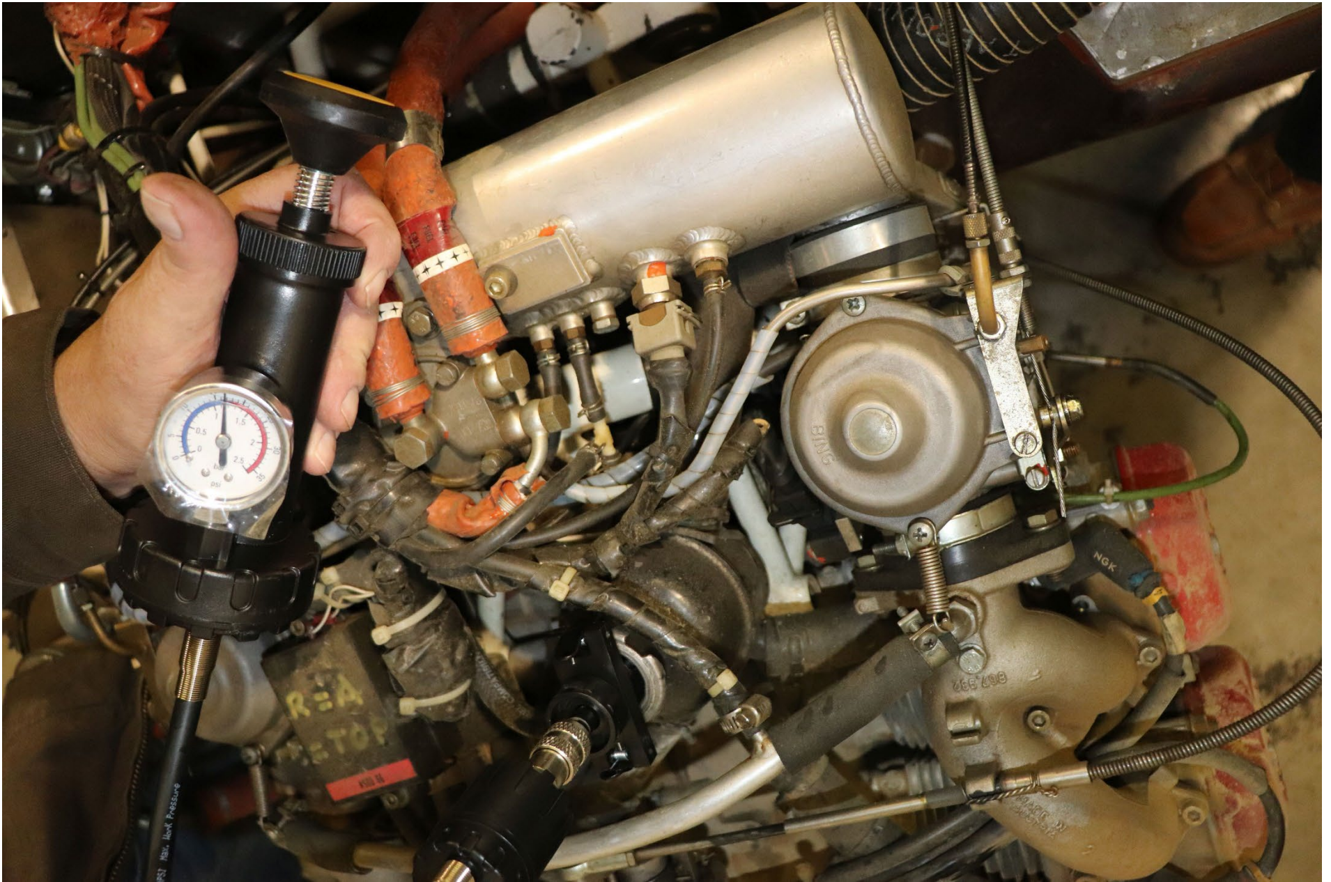
Photo 5 – View of engine during pressure test of cooling system
