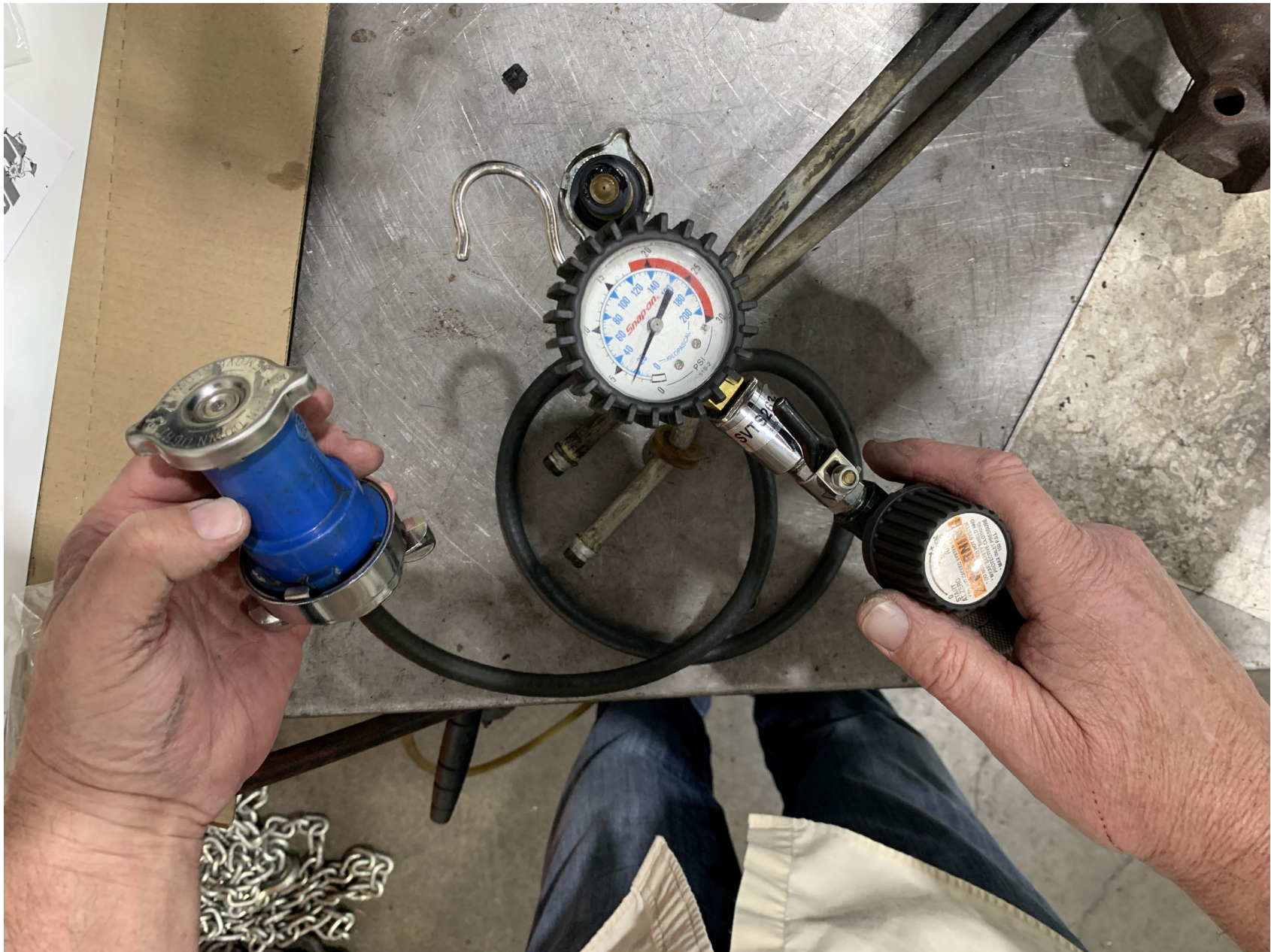
Photo 8 – View of pressure leak test of non-genuine Rotax radiator cap
