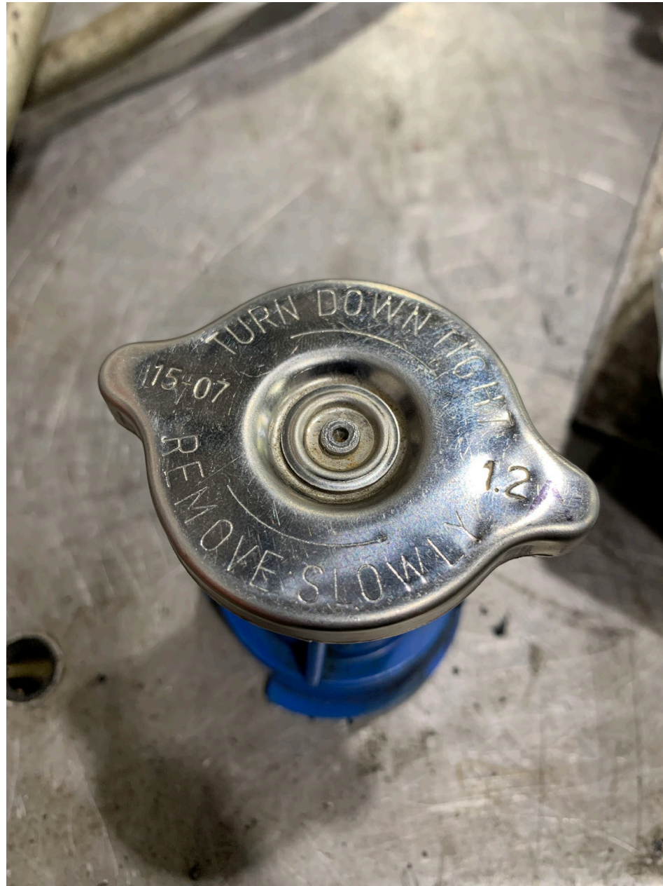
Photo 7 – View of non-genuine Rotax radiator cap installed on pressure leak test adapter
