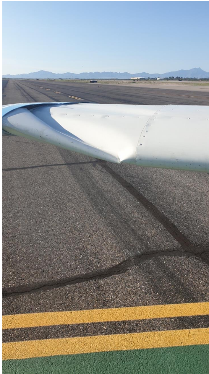
Photo 4 – Accident airplane-right wing tip damage. (Photo courtesy of the pilot)
