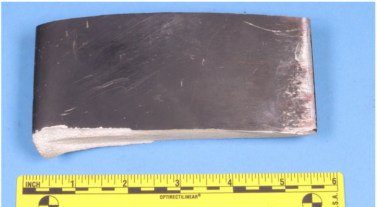
Figure 2 – View of the blade face surface of the propeller blade remnant, showing lack of paint and impact marks on the trailing edge (right in the figure).
