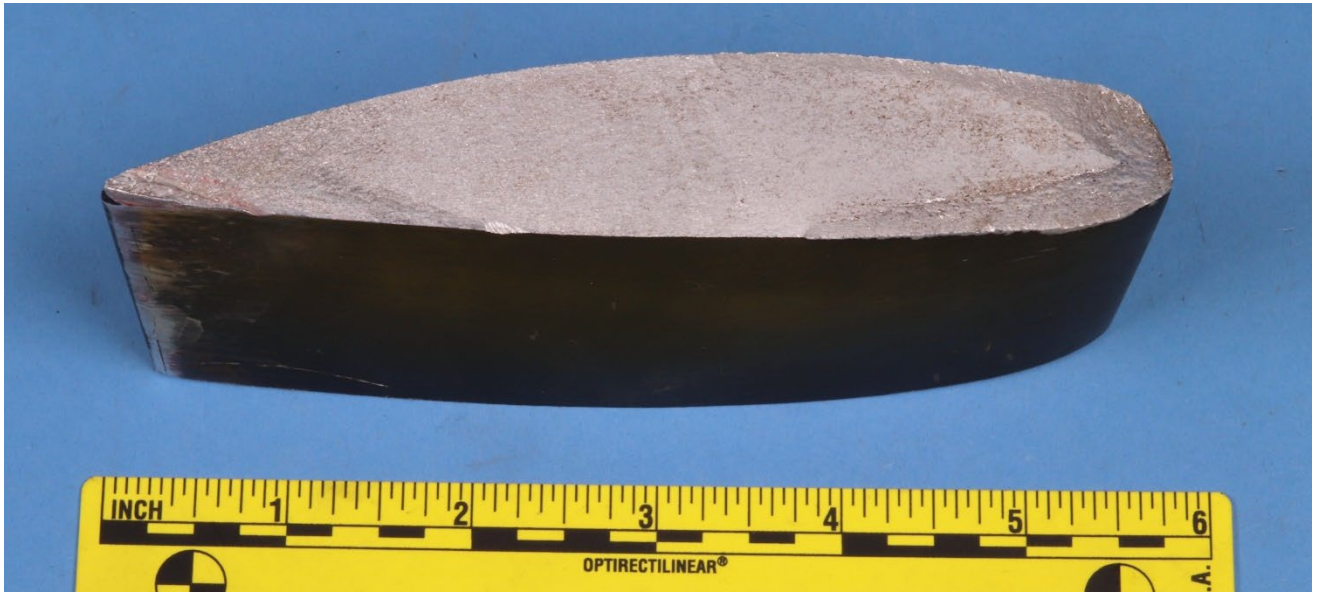
Figure 1 – Angled view of the propeller blade remnant, showing the fracture surface, as received.
