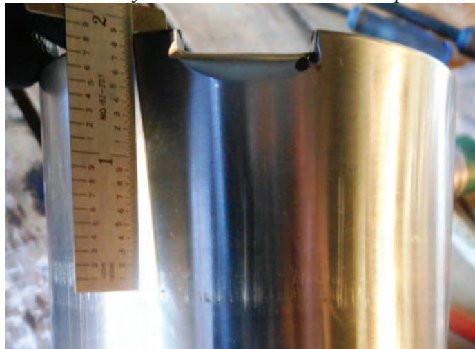
Photo #6 - Cylinder mark at ~1.9 below top corner
