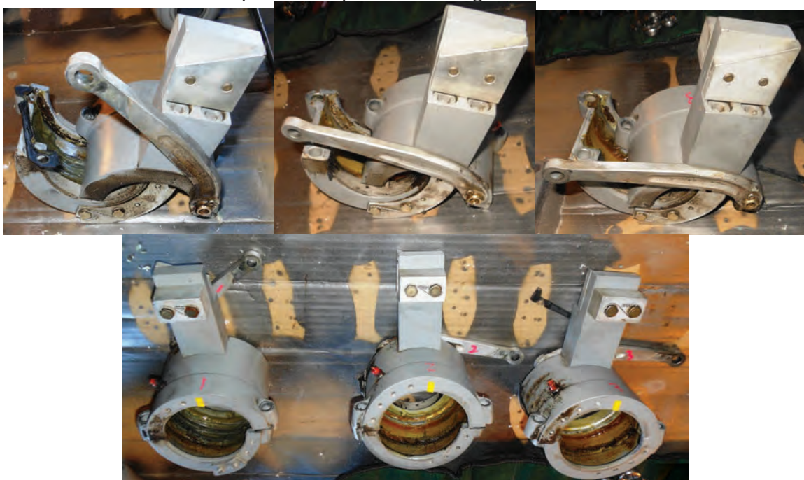
Photo #8 – Propeller clamps, counterweights and link screws/arms
