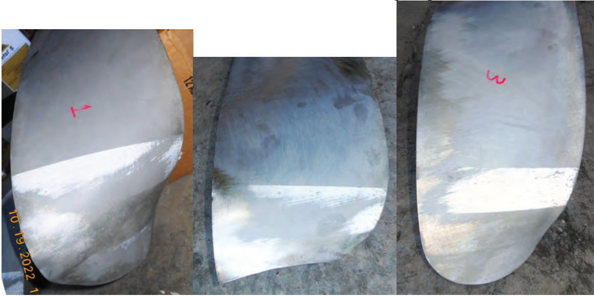
Photo #15 - Blade camber side near tip stripes
