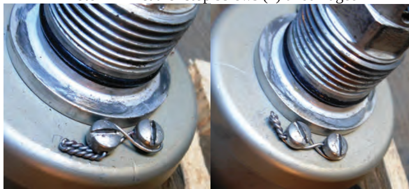
Photo #7 – Feather stop screws (4) undamaged
