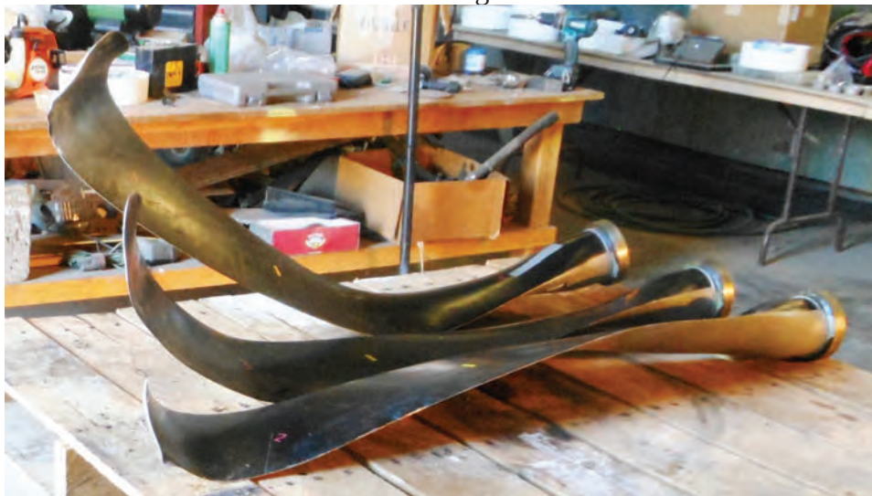
Photo #18 - Propeller blades trail edge view 2-3-1 (foreground to background) progressive bending
