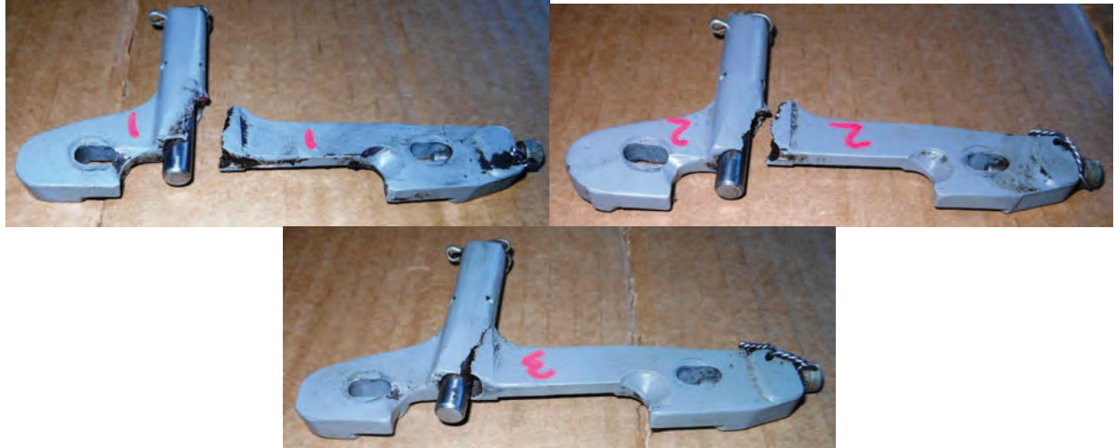
Photo #9 - Start lock brackets and plungers
