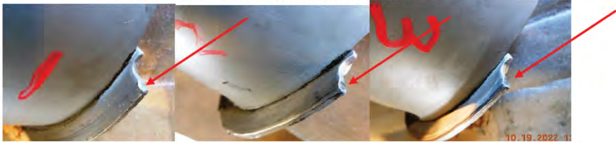
Photo #3 – Start lock plate - pin impact marks
