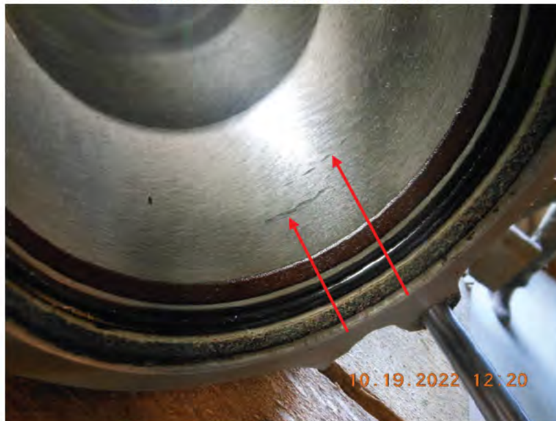
Photo #4 – Piston bore with marks
