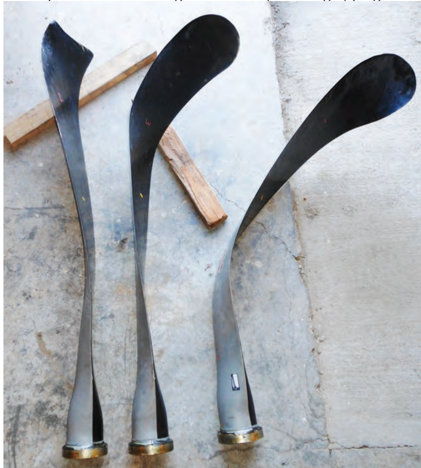
Photo #17 - Propeller blades trail edge view 2-3-1 (left-to-right) progressive bending
