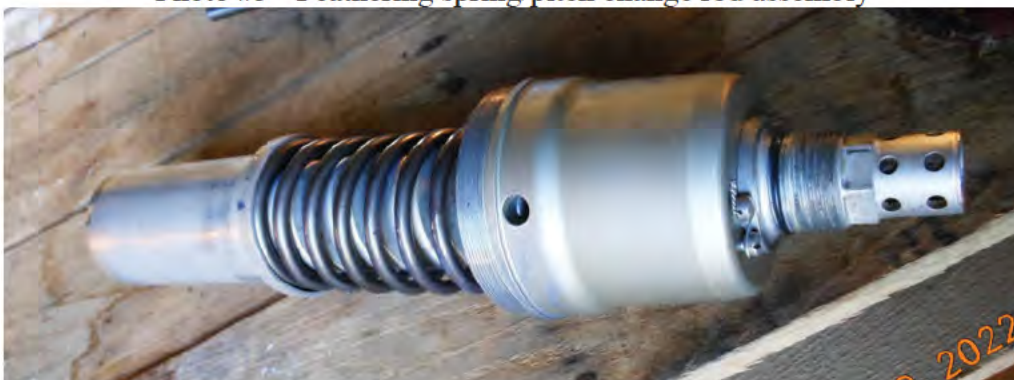
Photo #5 - Feathering spring/pitch change rod assembly
