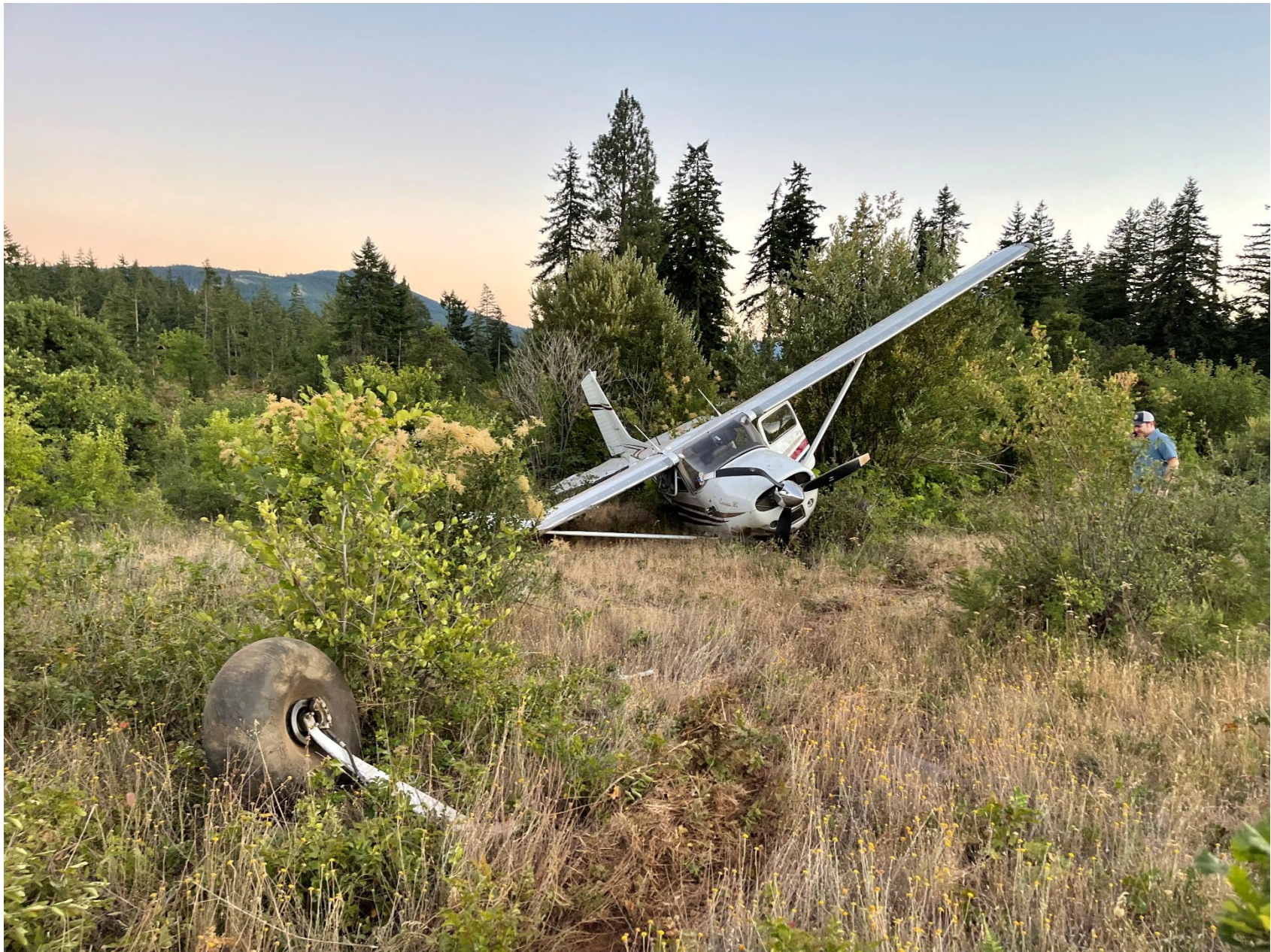
Photo 2 – N8884 front-right view, showing the right landing gear assembly. Photo courtesy of the pilot.
