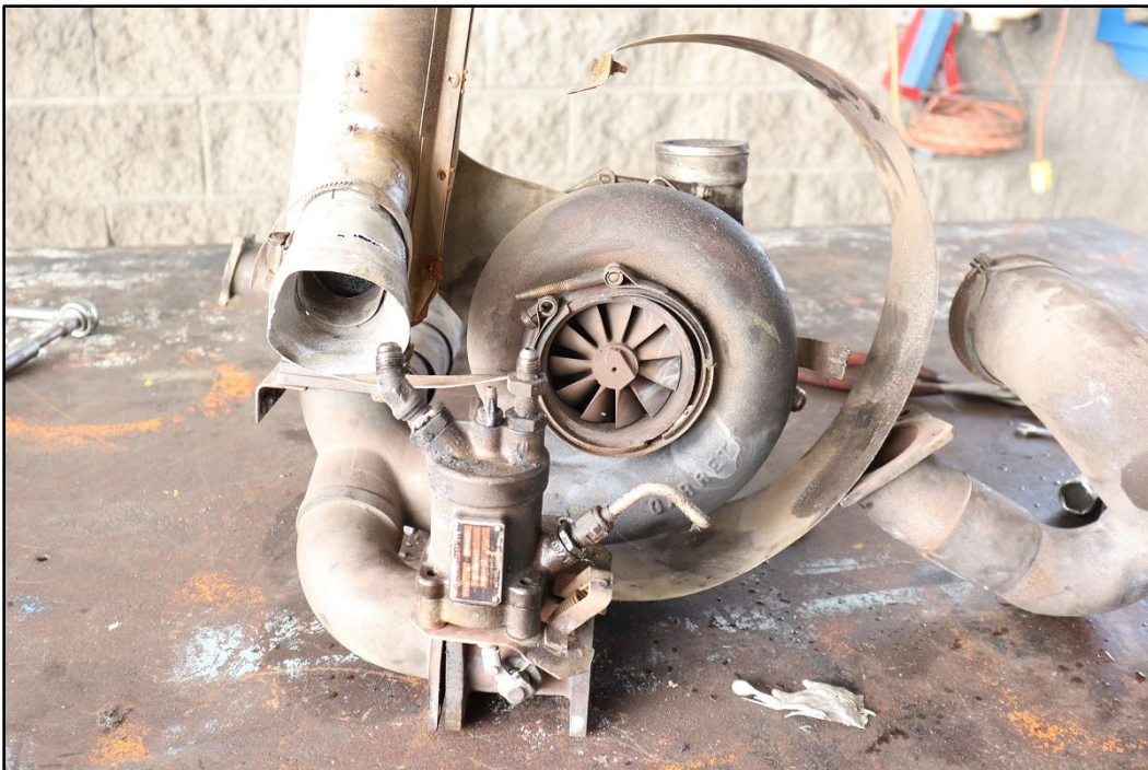
Figure 4: View of Turbo Charger, Photo Courtesy NTSB
