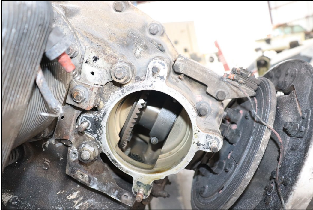
Figure 2: View of Alternator Port, Photo Courtesy NTSB
