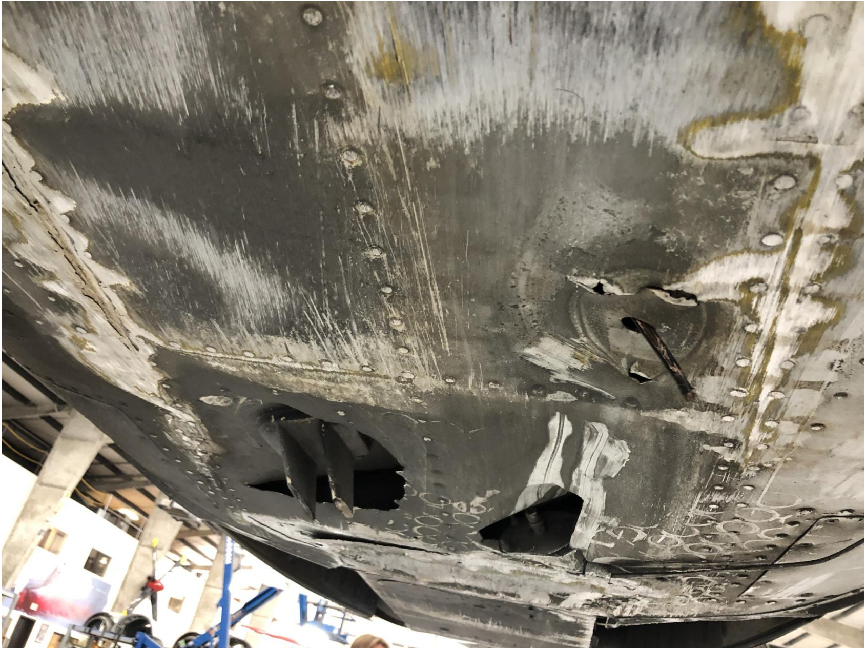
Photo 1 – View of airplane skin damage to lower fuselage (photo courtesy of the local fixed based operation)
