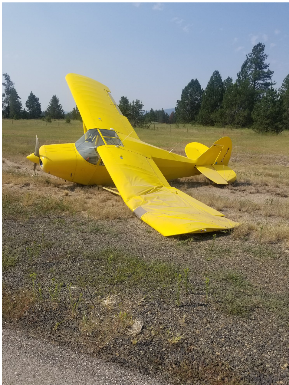
Photo 1 – View of left wing damage (Picture courtesy of owner)
