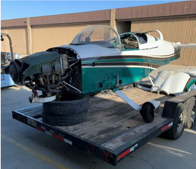
Figure 1: N468AC at storage facility, secured to a trailer for the engine test run
