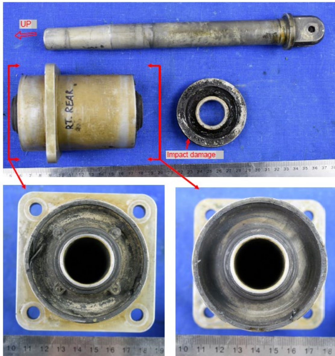
Figure 4. View of Right Aft Pylon Corner Mount
