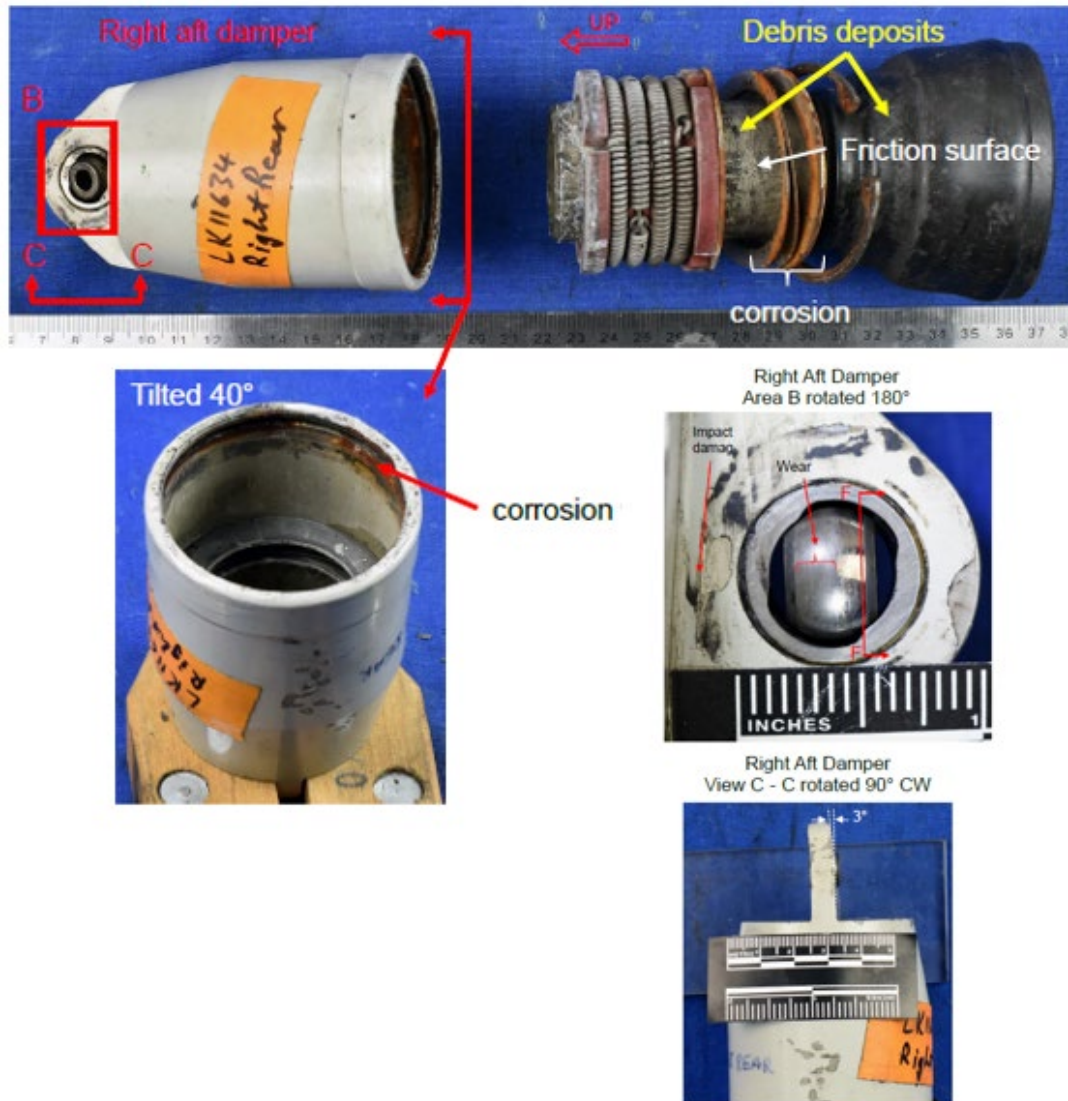
Figure 5. View of Right Aft Friction Damper
