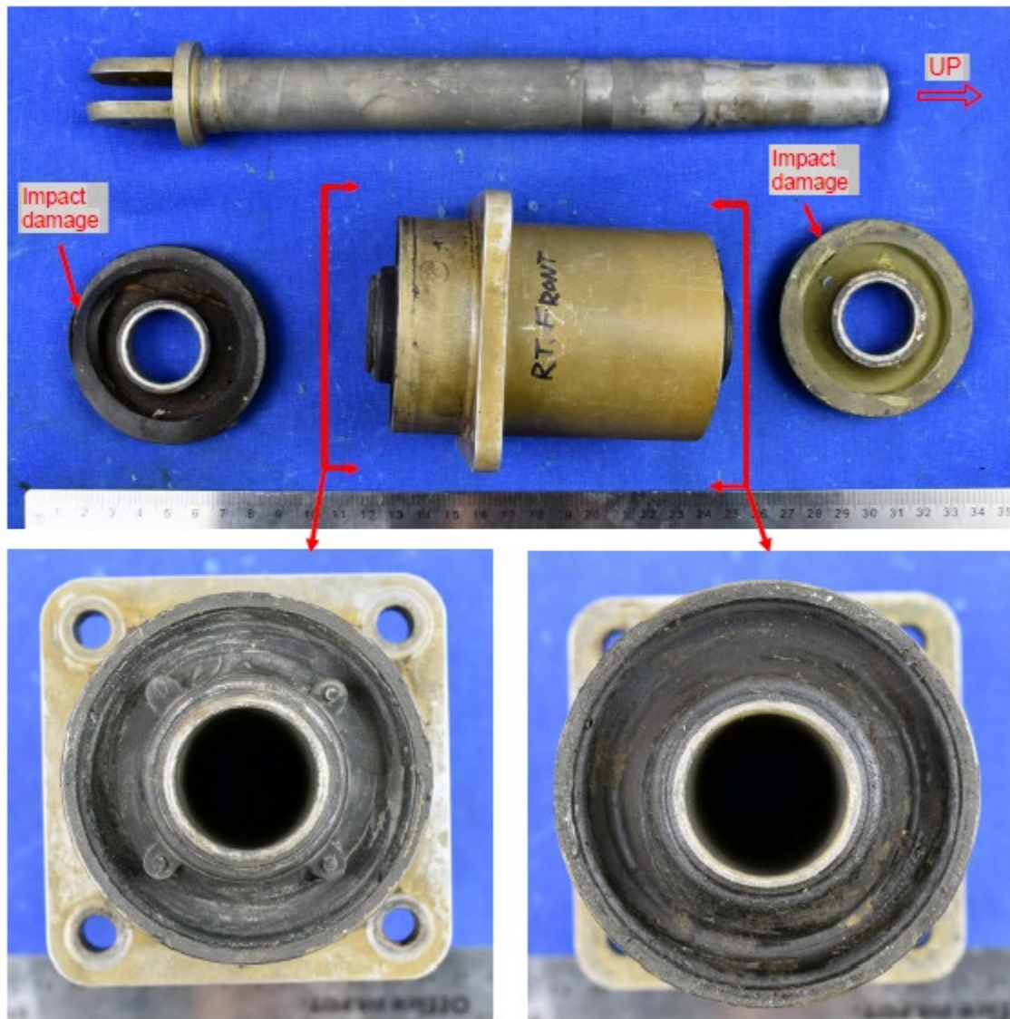
Figure 2. View of Right Forward Pylon Mount
