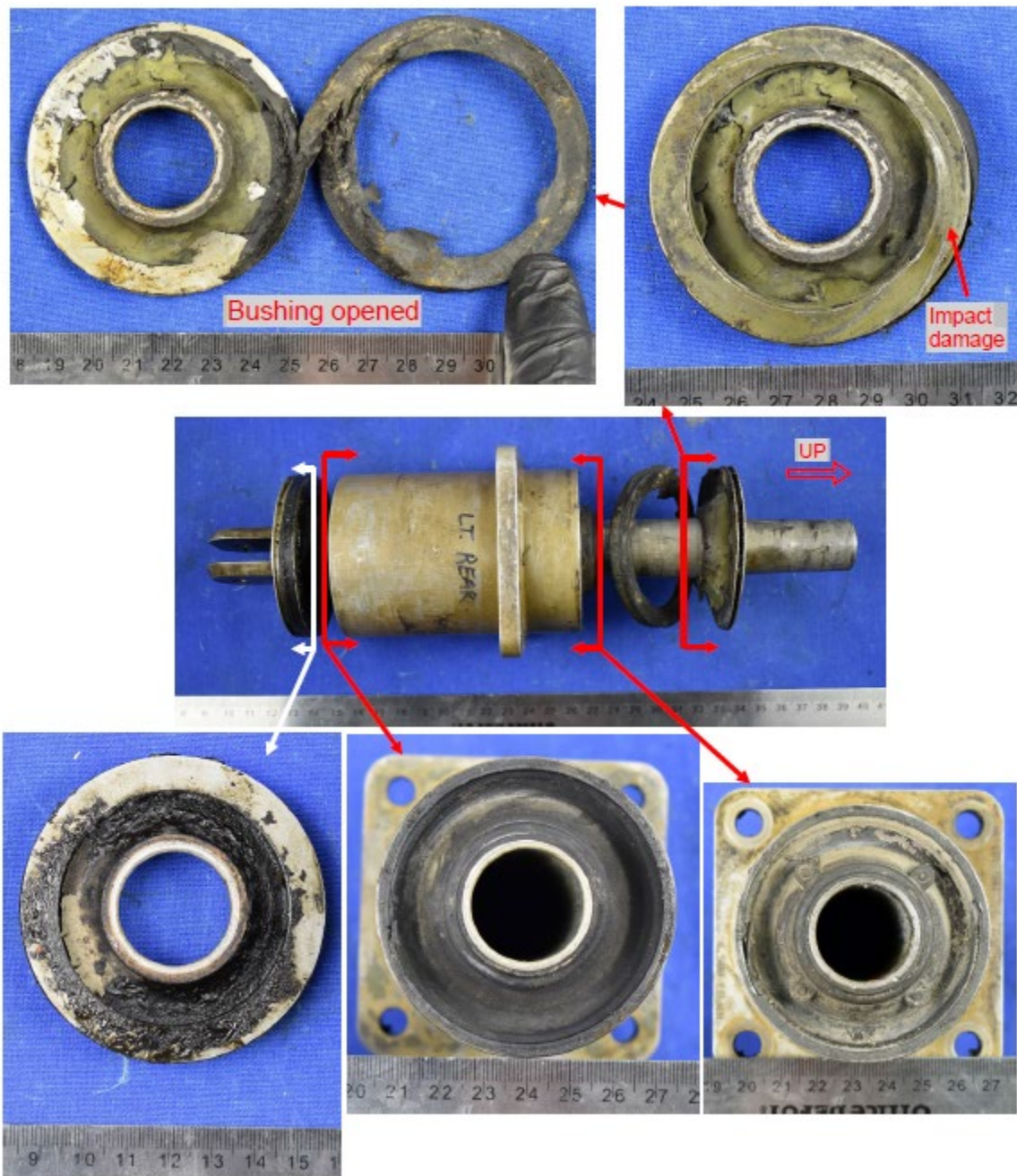
Figure 6. View of Left Aft Pylon Mount
