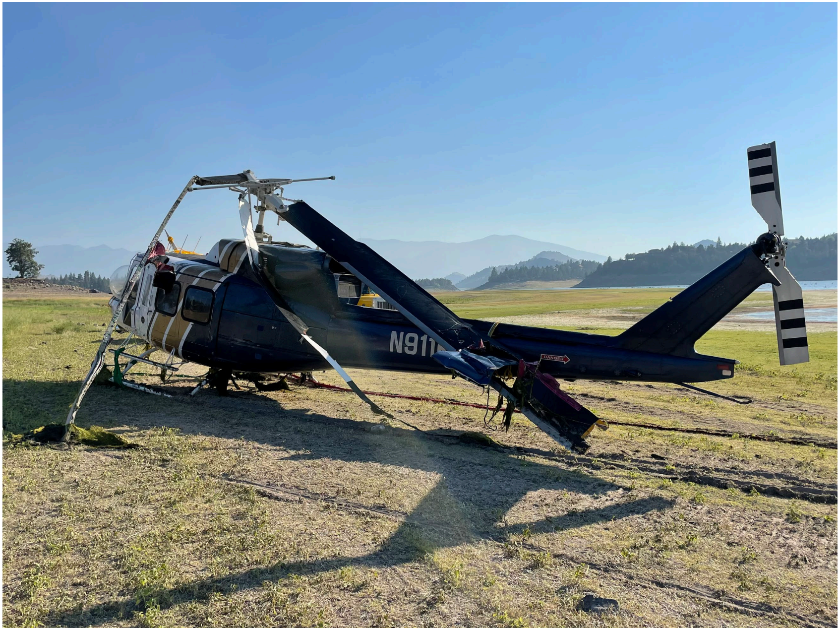
Photo 2 – View of recovered helicopter showing damage to rotor systems and fuselage (courtesy of recovery company)
