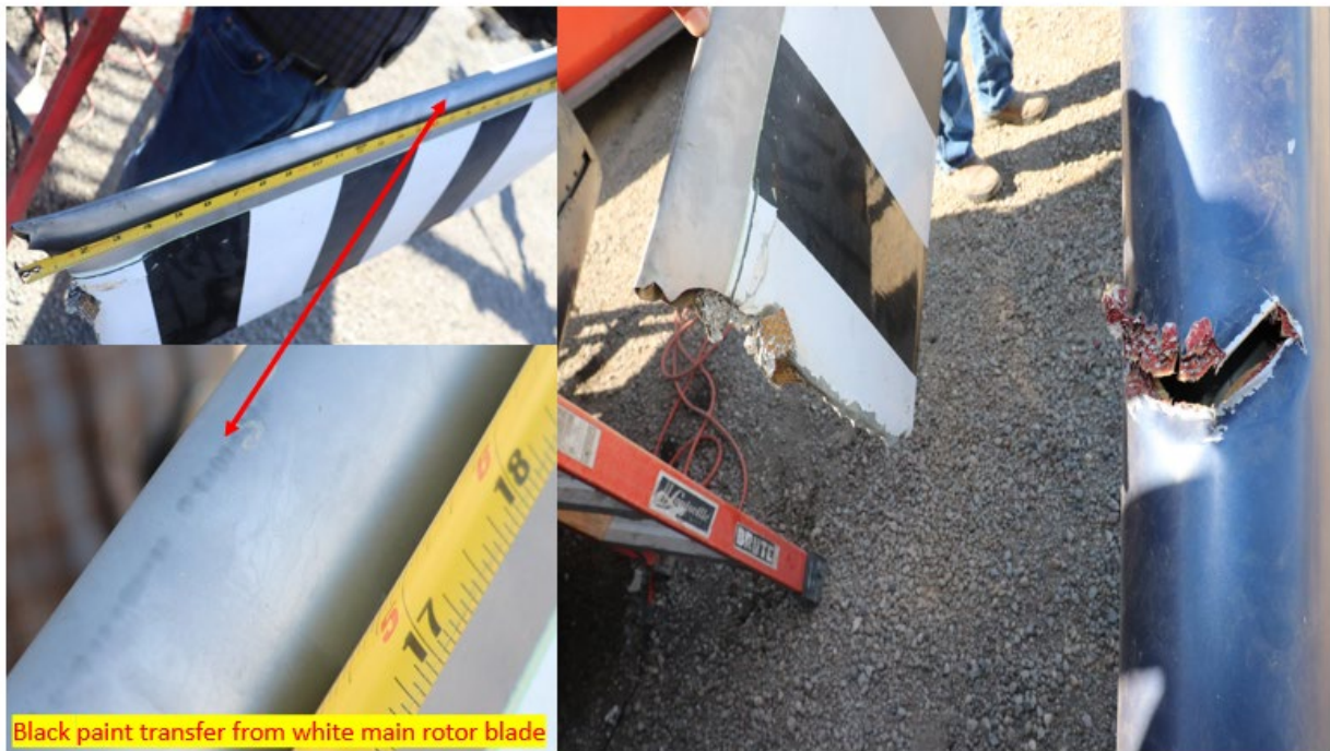
Figure 3. right photo: view of damage to vertical driveshaft cover and tail rotor blade; upper & lower left photos: view of close-up views of damage to leading edge
