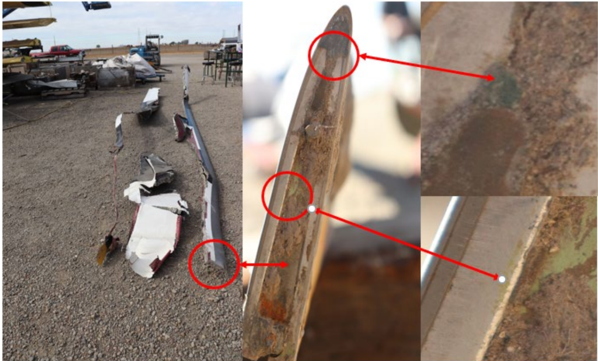
Figure 5. Left photo: view of white main rotor blade; middle and right photos: close-up views of outboard section of leading edge with paint transfers
