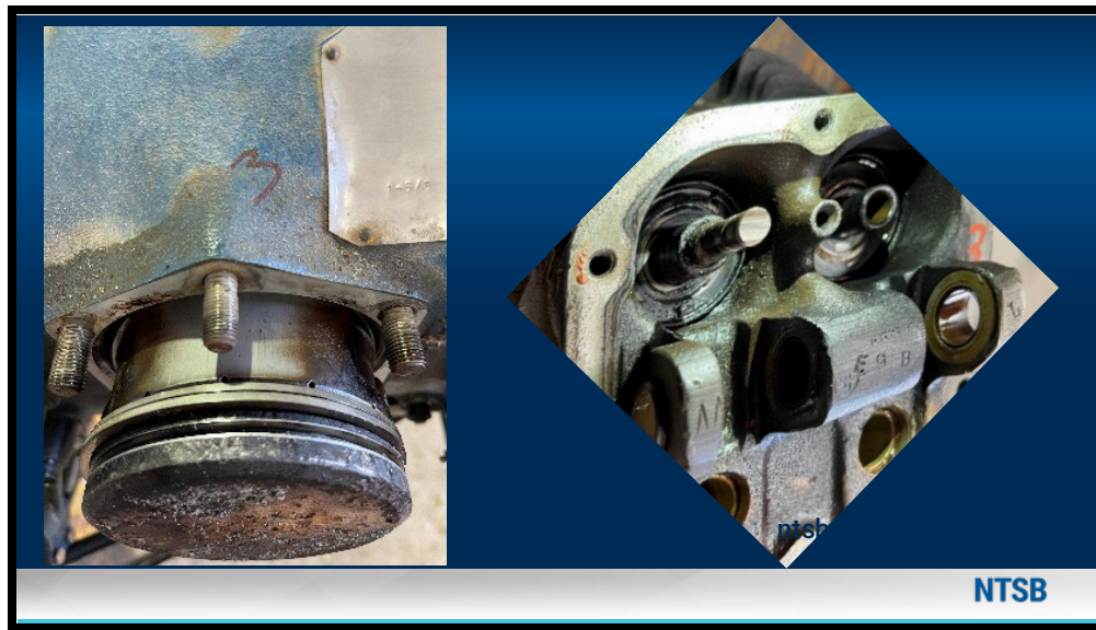
Figure 9: Images of No. 3 piston with missing top compression ring No. 3 cylinder stuck exhaust valve
