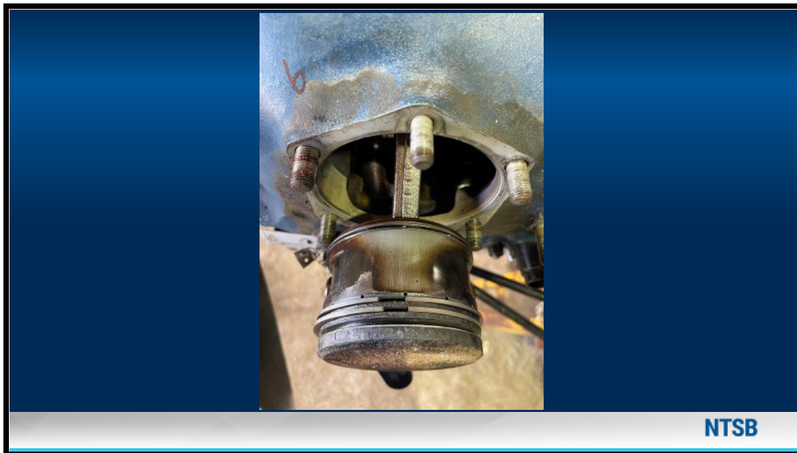
Figure 10: Image of No. 6 piston with missing top compression ring
