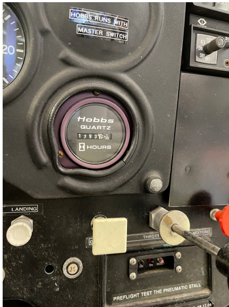
Photo 5 – View of N3871L Hobbs meter during examination, indicating 1,793.7 hours (Courtesy of IIC)
