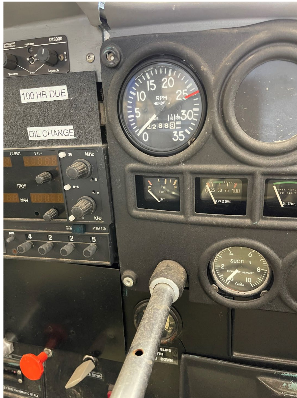
Photo 4 – View of N3871L engine tachometer reading during examination, indicating 2,288.8 hours (Courtesy of IIC)
