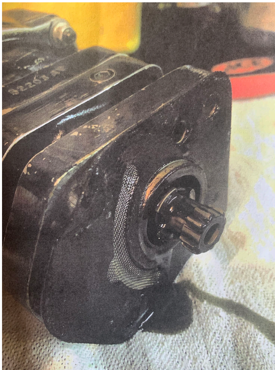
Photo 3 – View of propeller governor drive gear (View of propeller governor gasket (courtesy of Wings West Exchange & Overhaul, Inc))
