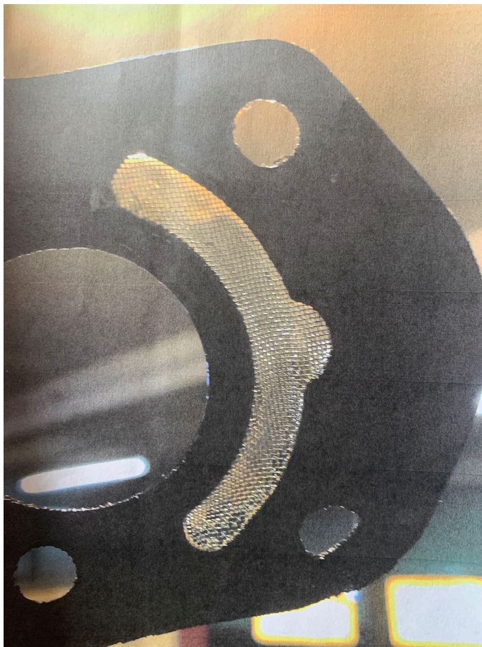
Photo 4 – View of propeller governor mounting gasket (courtesy of Wings West Exchange & Overhaul, Inc)
