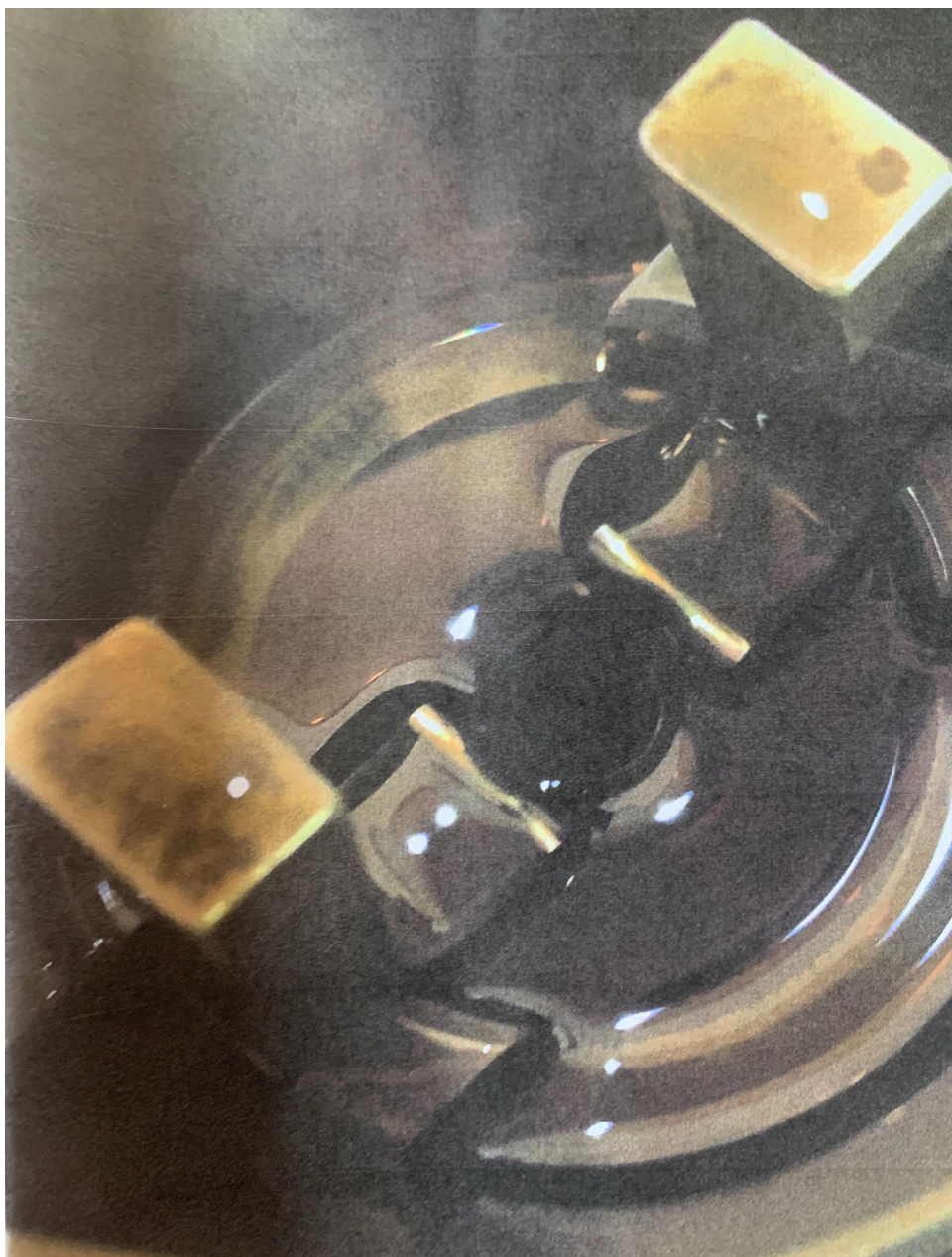
Photo 2 – View of propeller governor fly weights (courtesy of Wings West Exchange & Overhaul, Inc)
