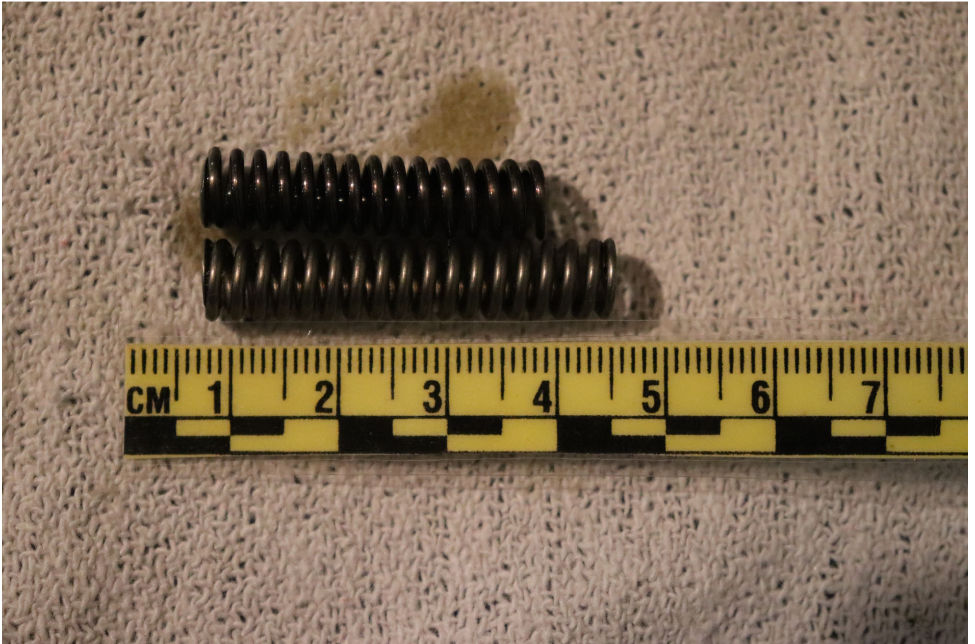
Photo 6 – Comparison in length of relief valve springs. Upper spring is the removed spring, and the lower spring is an exemplar spring (courtesy of Wings West Exchange & Overhaul, Inc)
