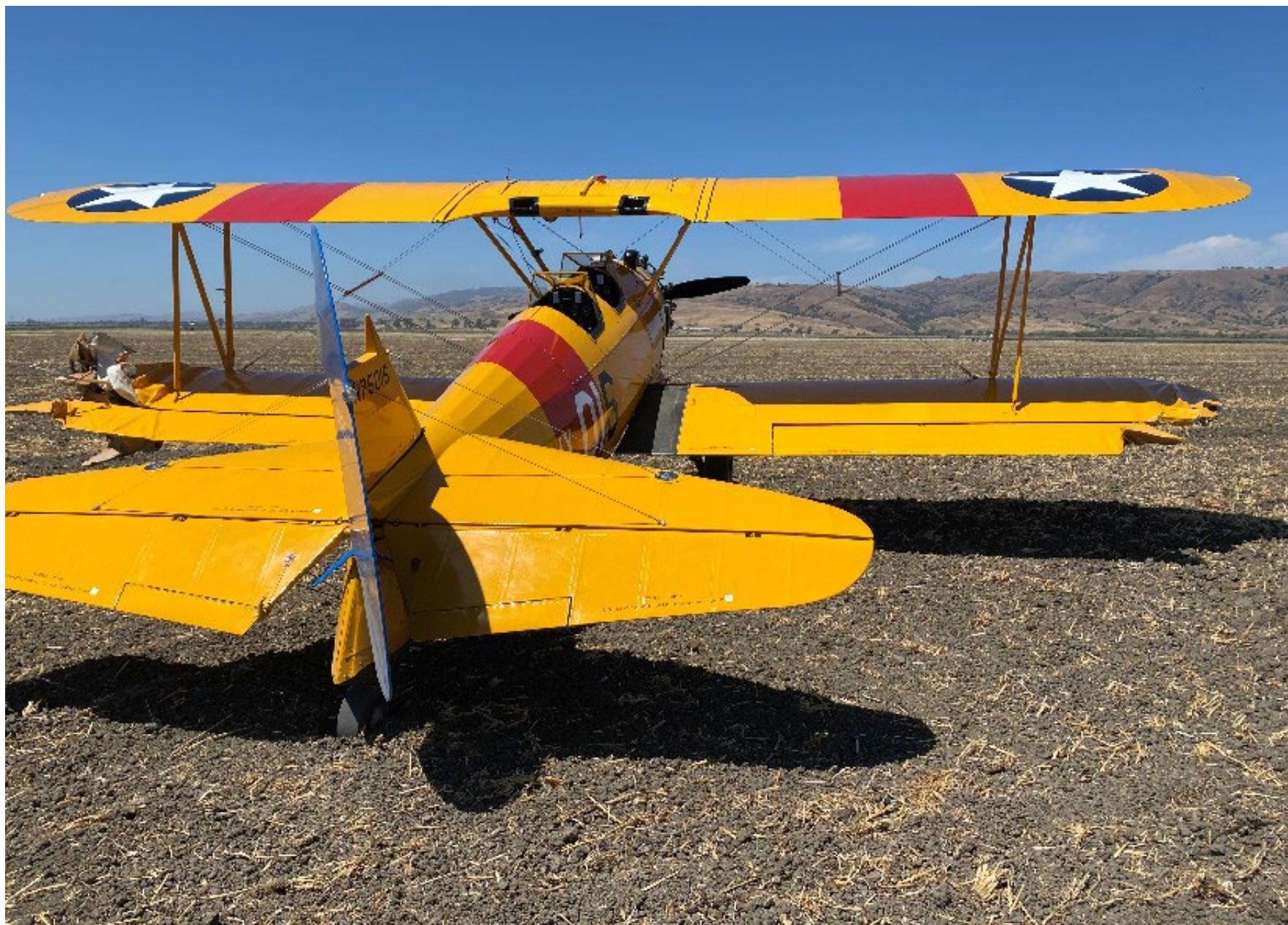
Photo 1 – View of airplane with damage to both lower left and right lower wings (courtesy of the pilot)
