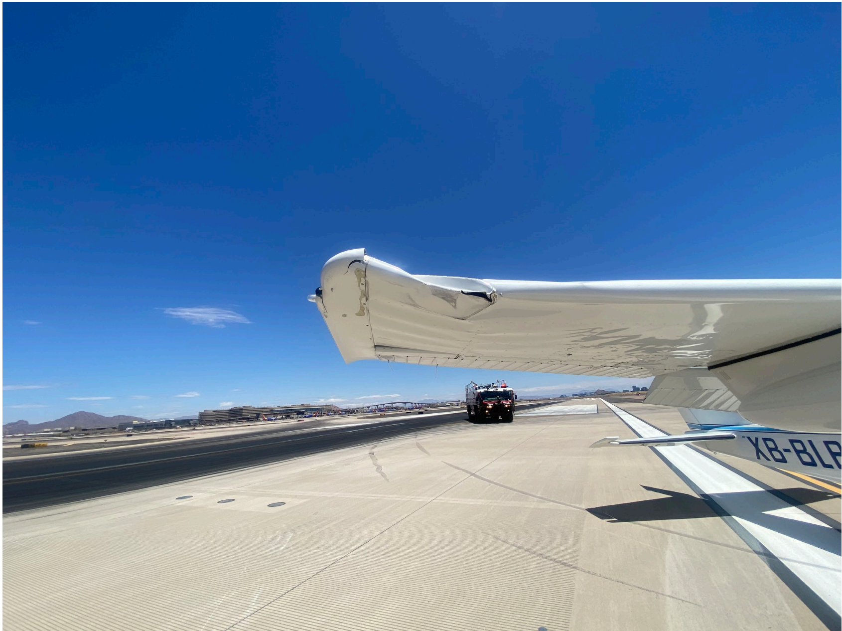
Photo 1 – View of right wing damage (photo courtesy of airport operations)
