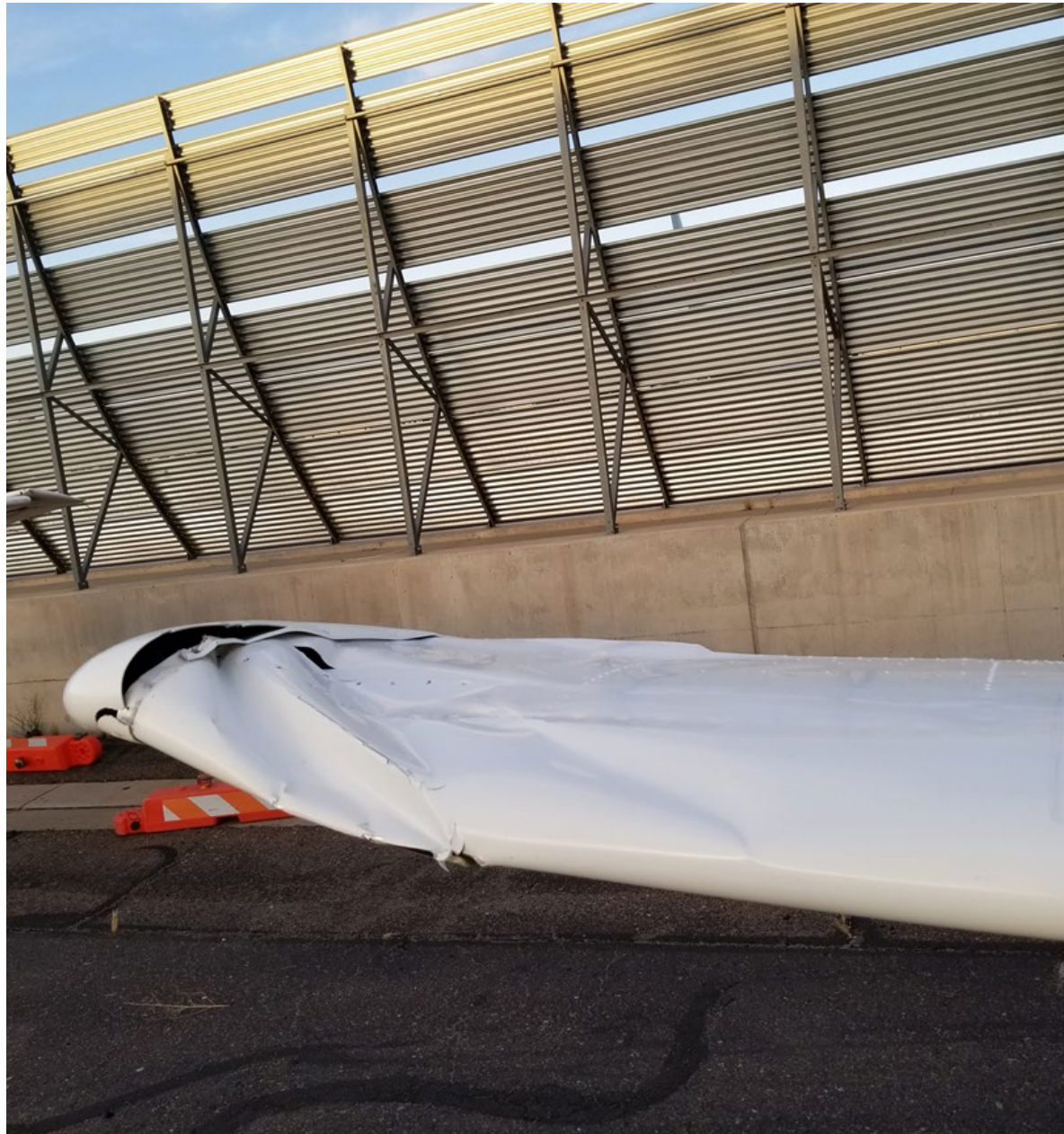
Photo 2 - View of right wing damage (photo courtesy of airport operations)
