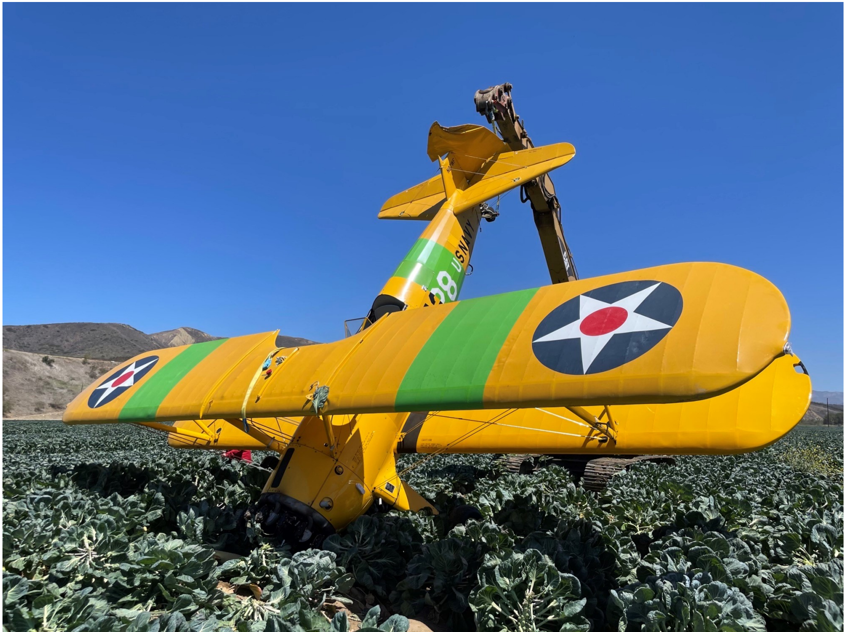
Photo 1 –N87WF with substantial damage to the rudder. Photo courtesy of the pilot.
