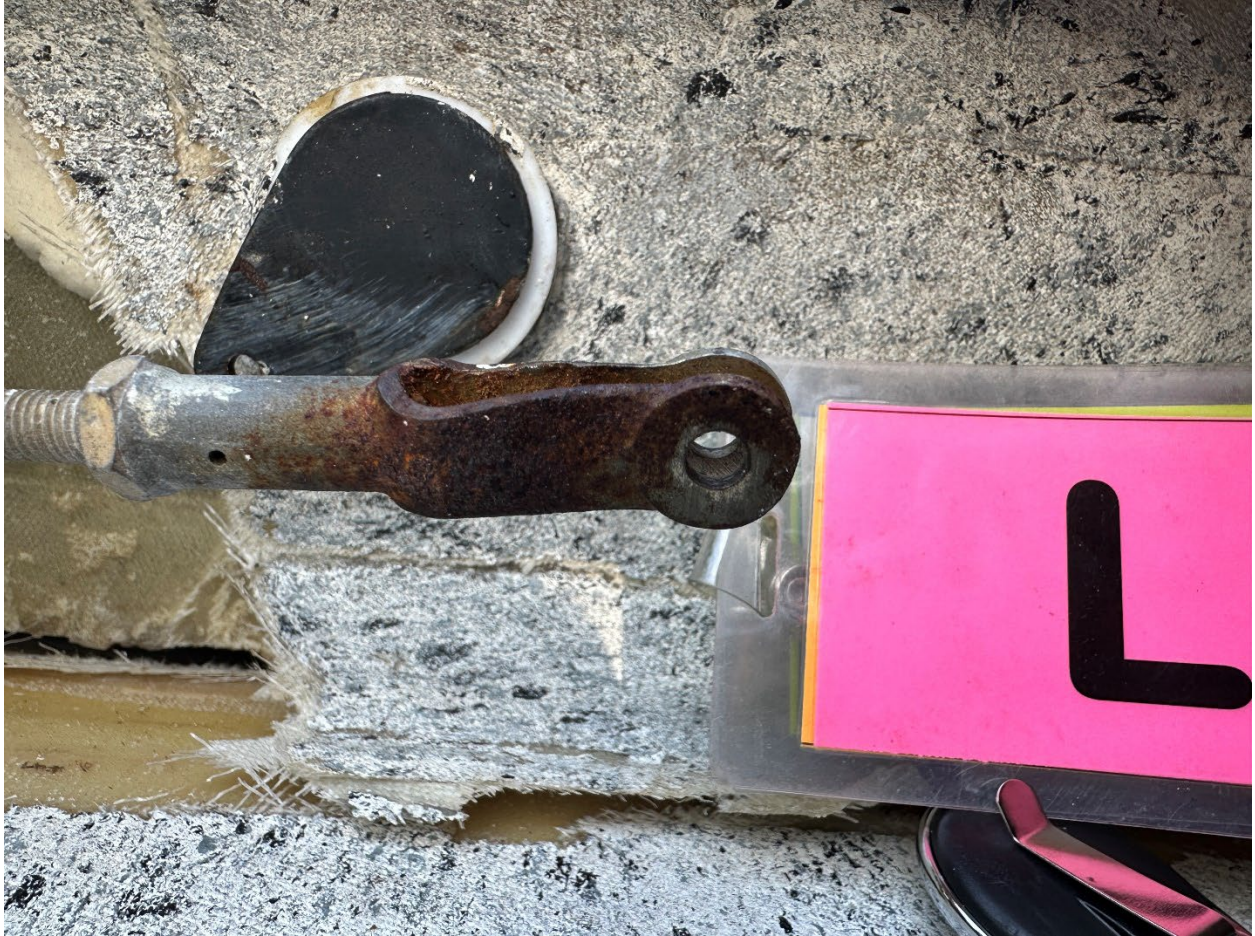
Figure 3. Detached left wing flap hardware welded plate and turnbuckle fork
