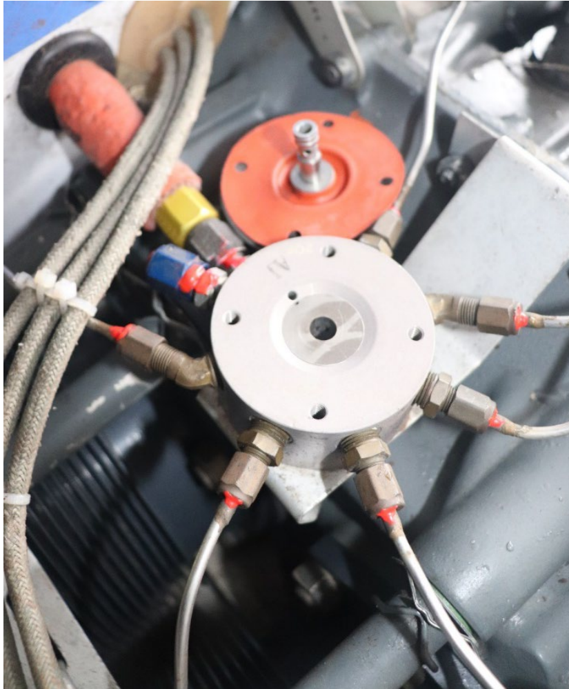
Figure 4. A close-up picture of the fuel flow divider showing diaphragm
