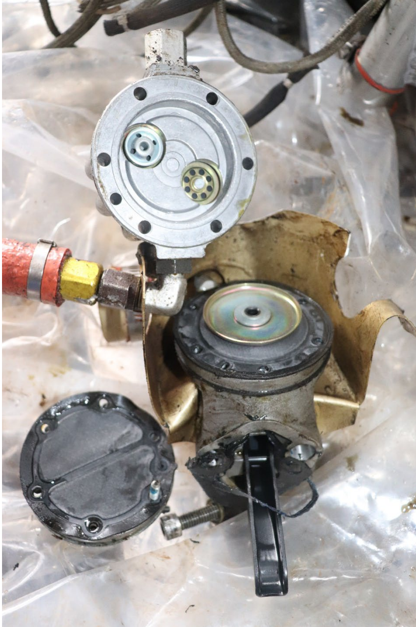
Figure 6. A picture of the disassembled fuel pump
