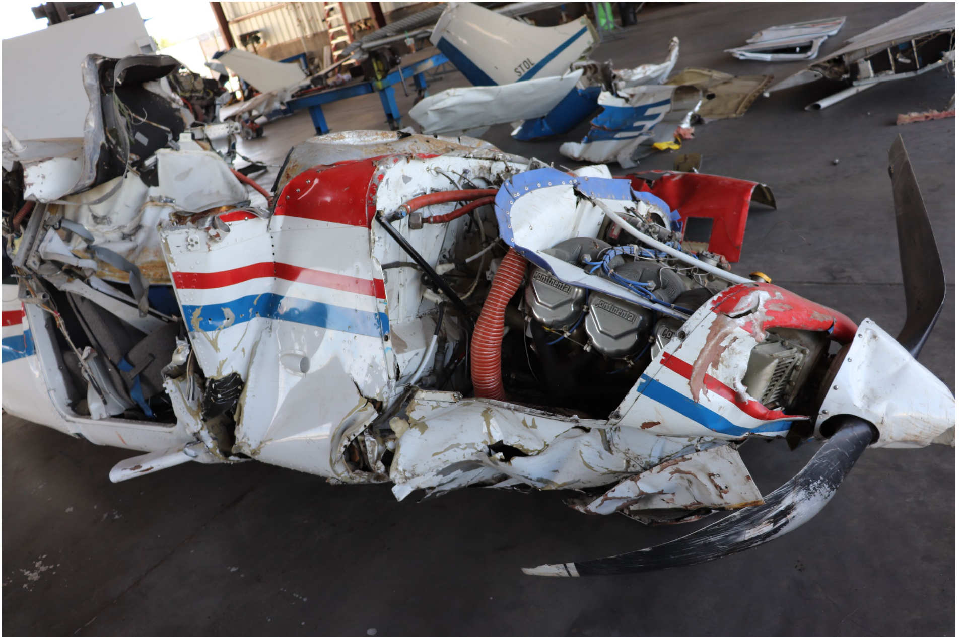
Photo 4 - Right side view of fuselage damage (photo courtesy of the NTSB)
