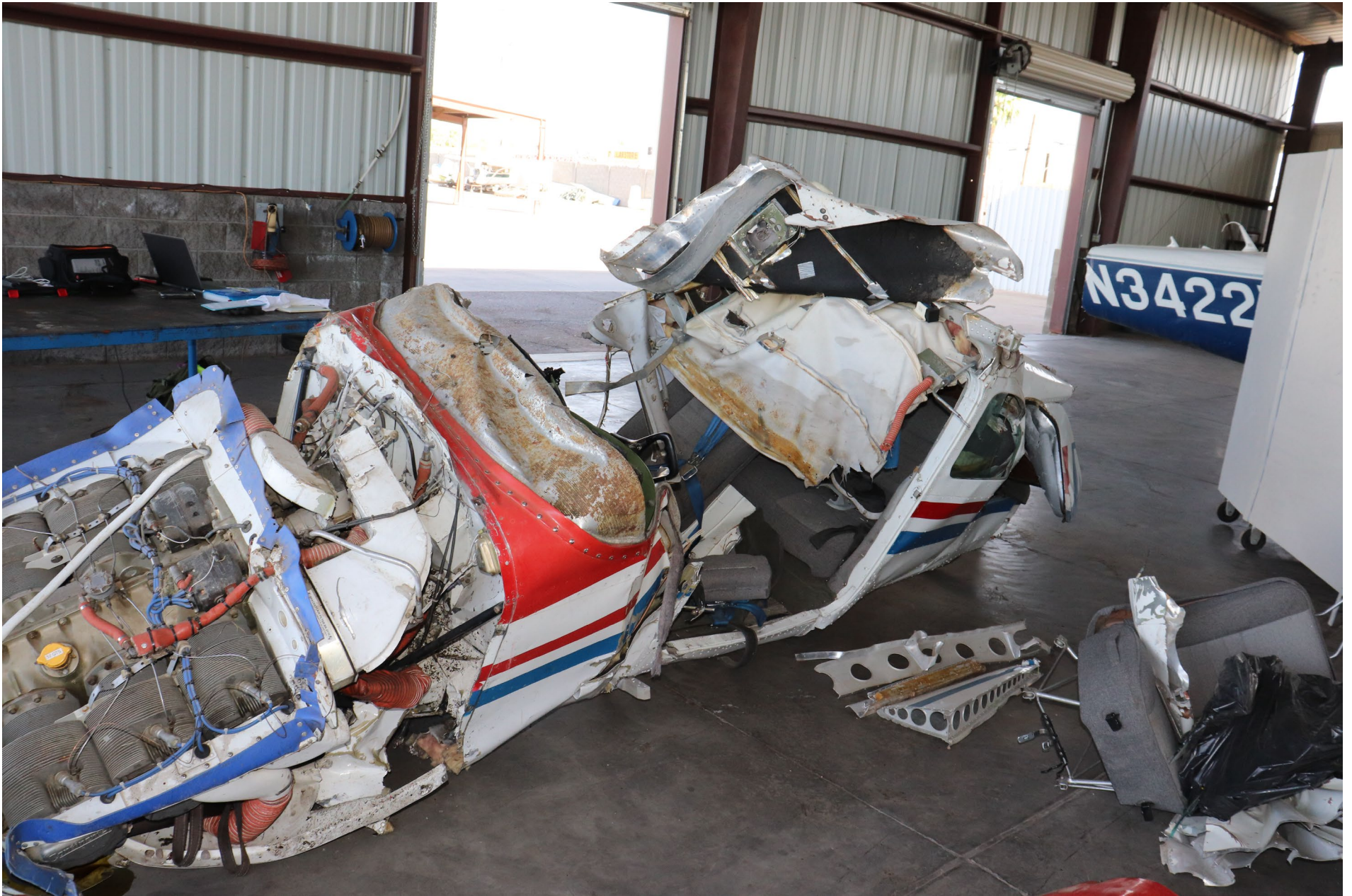
Photo 2 - Left side view of fuselage damage (photo courtesy of the NTSB)
