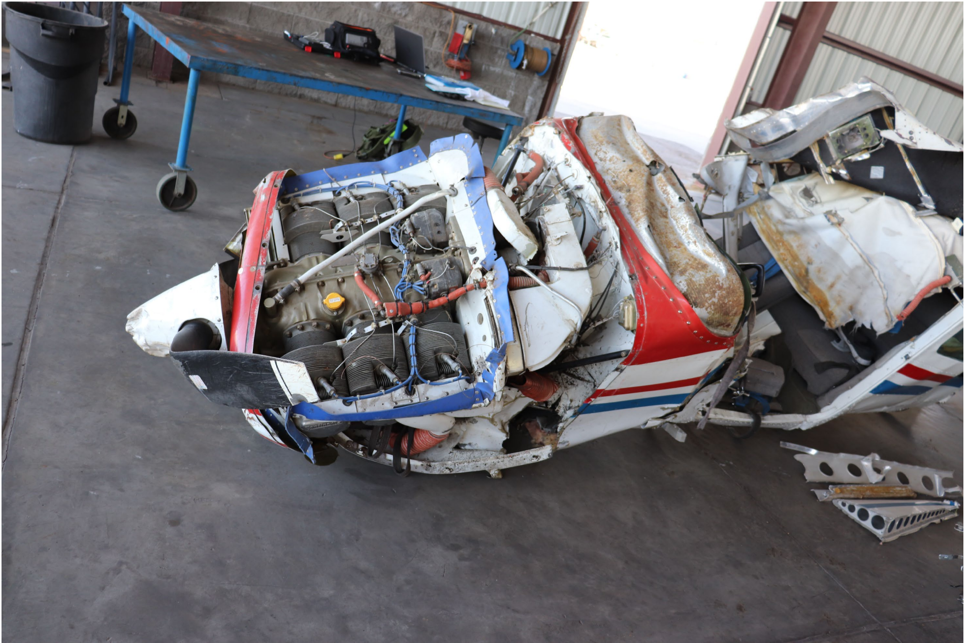
Photo 1 – Left side view of fuselage damage (photo courtesy of the NTSB)
