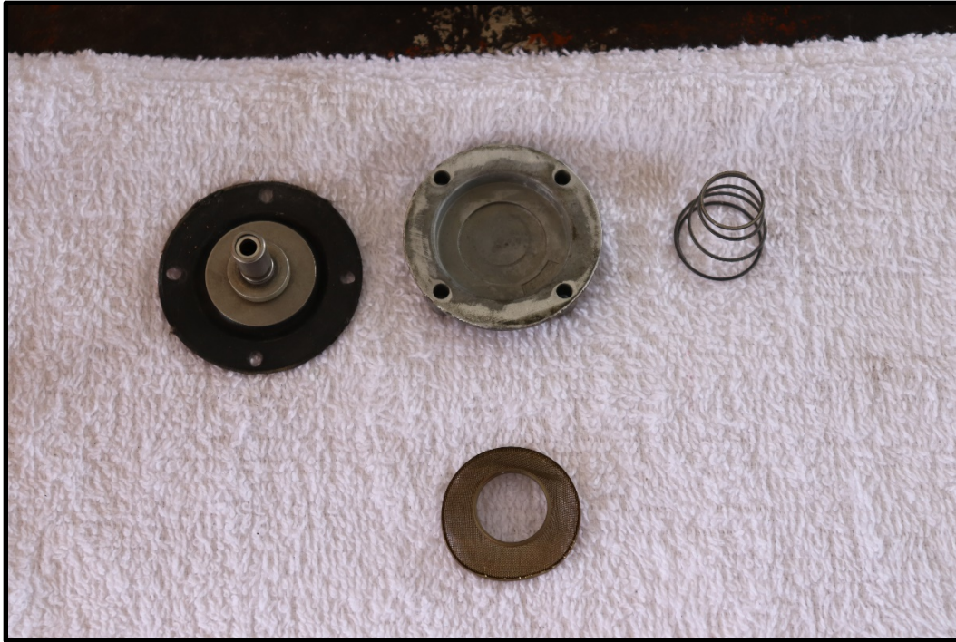
Figure 9: View of fuel flow manifold spring and diaphragm
