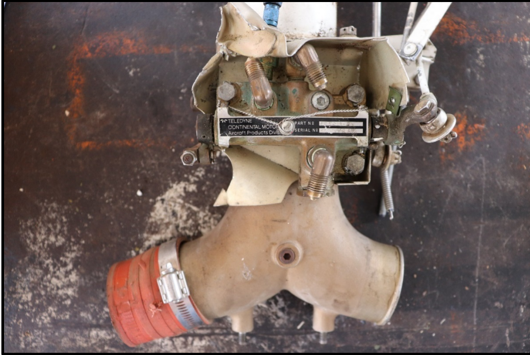
Figure 7: View of throttle body
