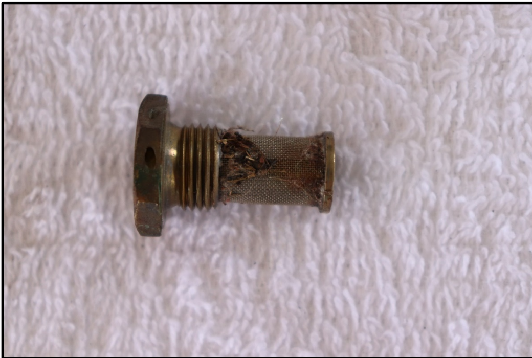
Figure 8: View of debris on fuel inlet fuel screen
