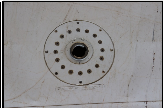
Figure 3. View of left fuel filler port
