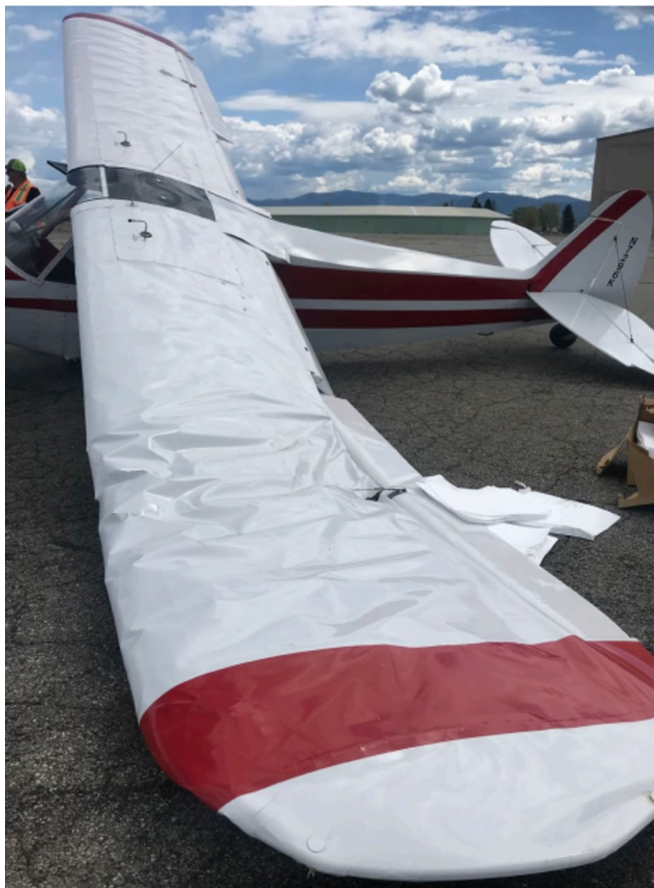
Photo 1 – N7296K, showing damage to the left wing. Photo courtesy of the pilot.
