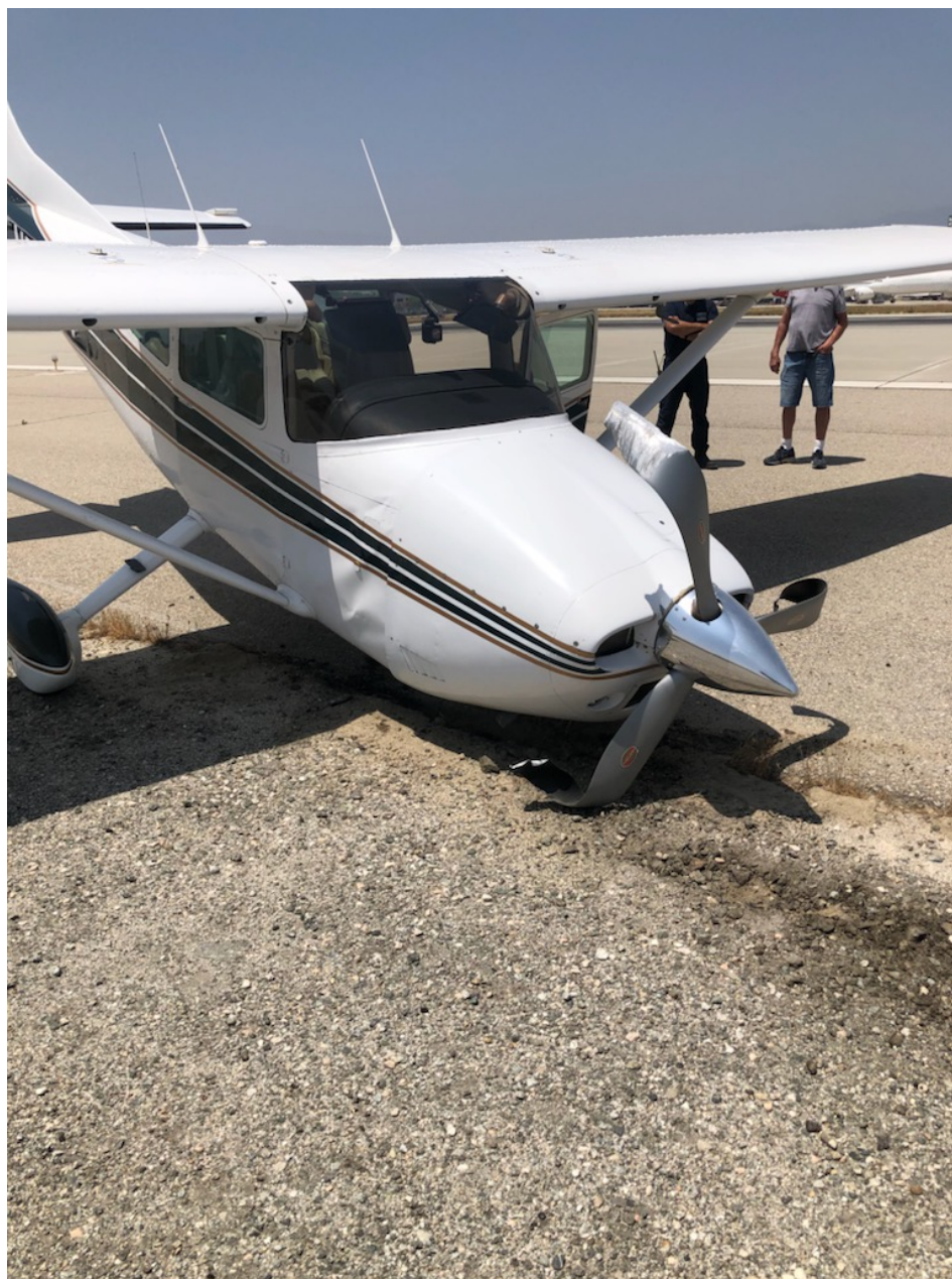
Photo 1 – View of fuselage damage aft of the firewall (photo courtesy of the pilot)
