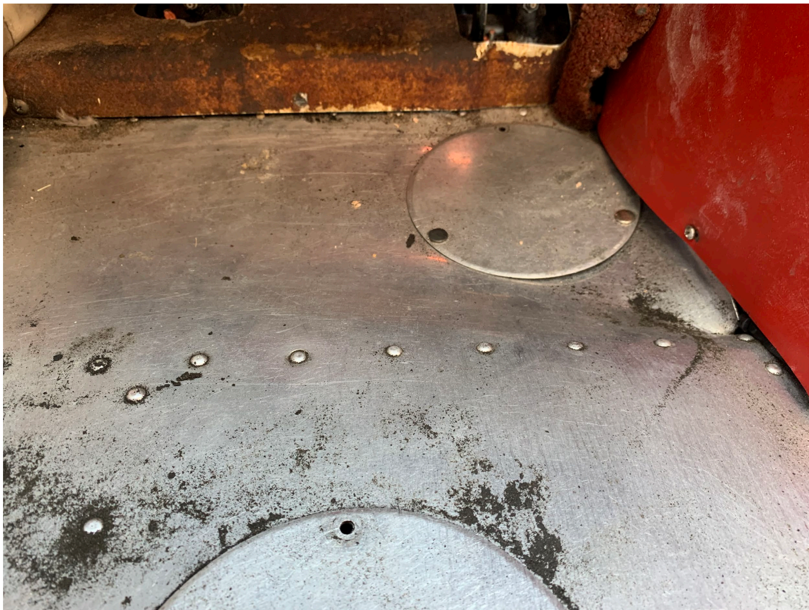
Photo 2 – Buckling at pilot seat foot well (Courtesy of Federal Aviation Administration)
