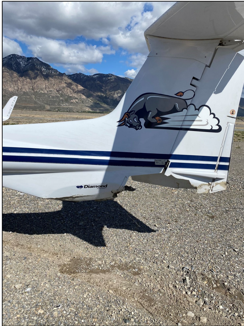
Photo 1 – View of rudder damage (photo courtesy of the flight instructor)
