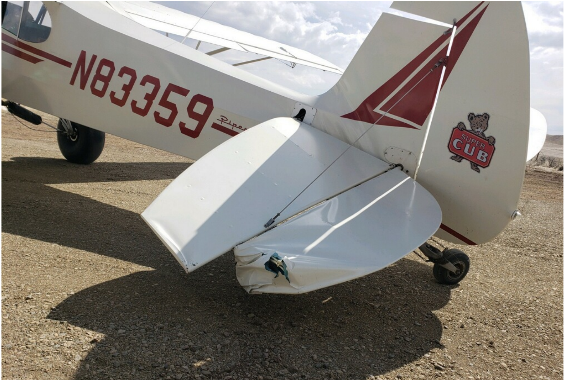
Photo 2 – N83359 Left Elevator Damage, courtesy owner
