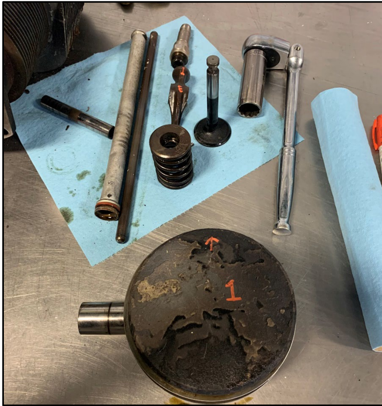
Figure 2: View of No. 1 piston head and disassembled components for No.1 cylinder valve train.
