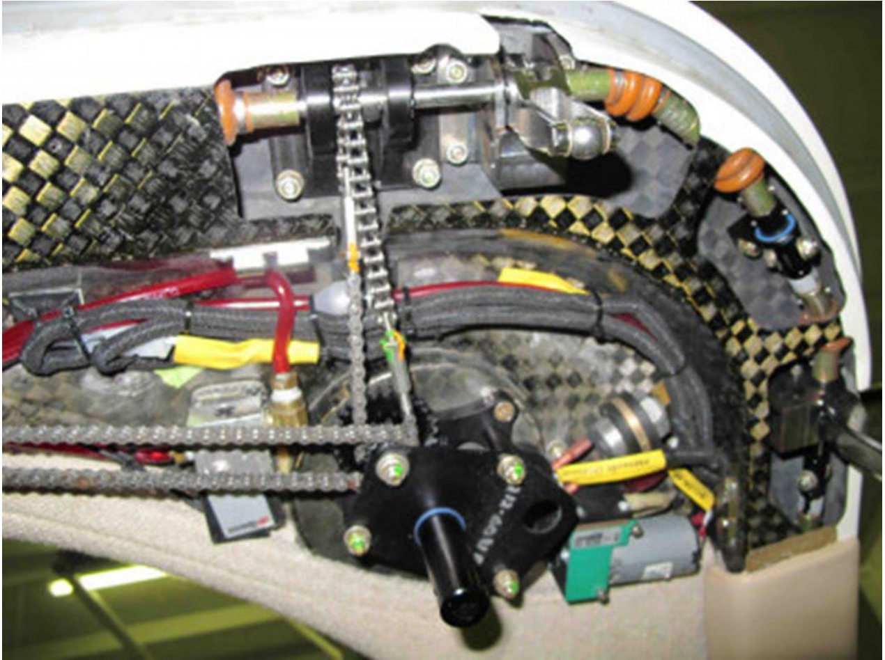
Latch system (above). Above photo is of an earlier Evolution kit.
