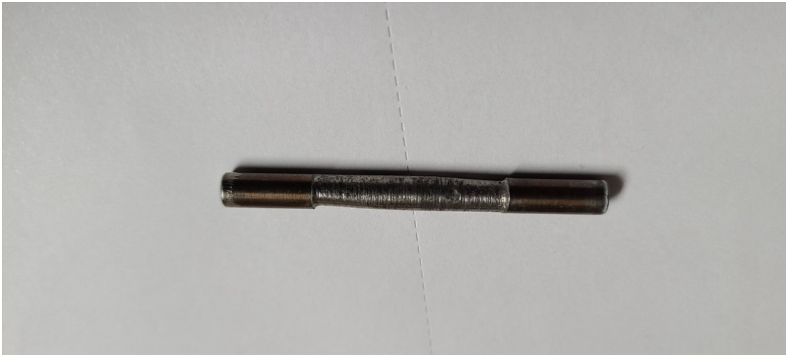
Worn hinge pin pictured.
