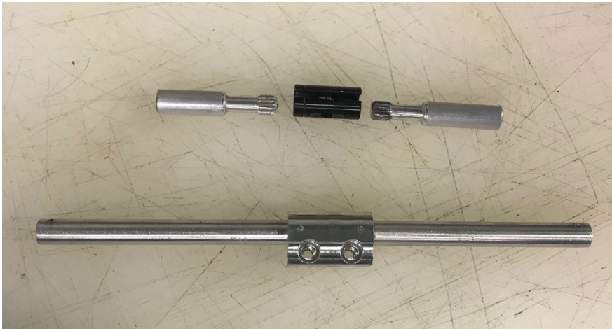
Original spline drive pictured on top. Current, preferred, coupler system on bottom.
