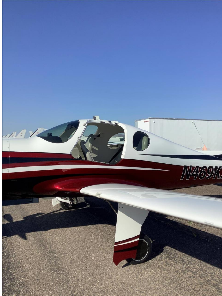
Photo 1 – Left side of airplane with missing door (Courtesy of Federal Aviation Administration)
