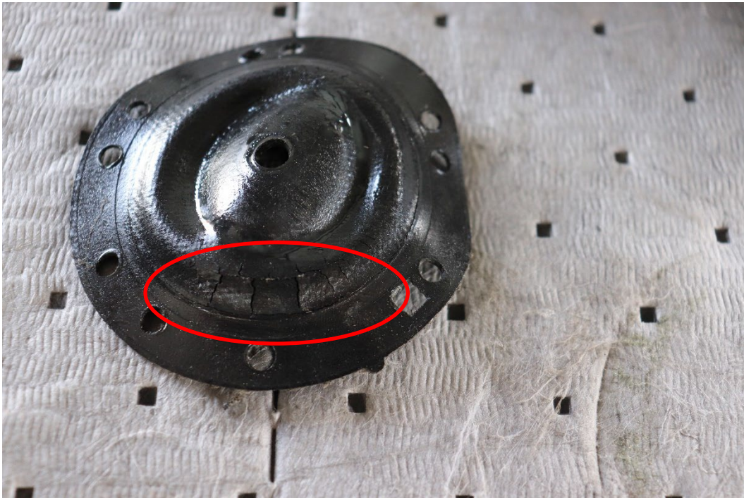
Figure 4: View of oil diaphragm with cracking (photo courtesy of the NTSB)
