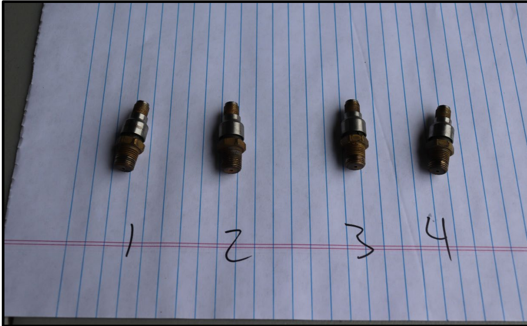
Figure 8: View of fuel injector nozzles (photo courtesy of the NTSB)
