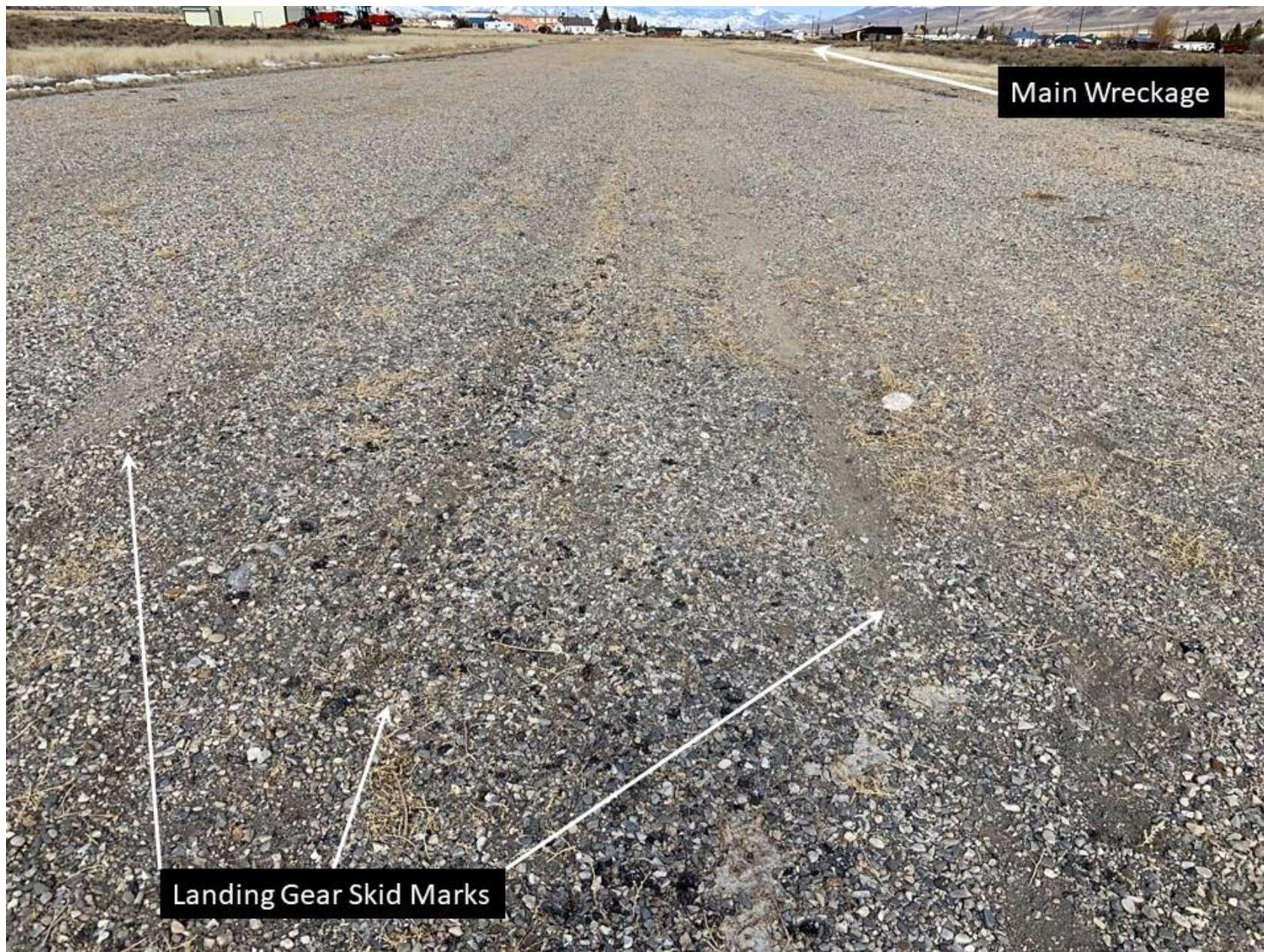
Photo 7 – Accident site, first identified contact with the runway. (Courtesy of the Lemhi County Sheriff's Office)
