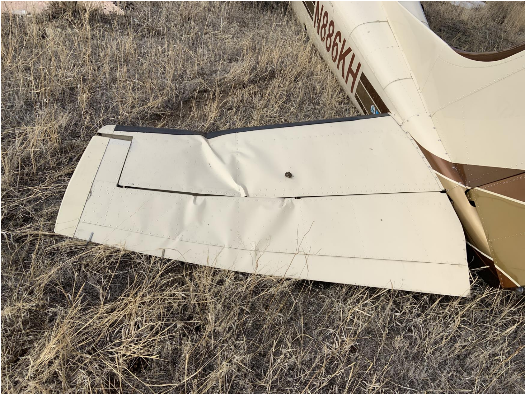
Photo 5 – Accident site, left horizontal stabilizer and elevator. (Courtesy of the Lemhi County Sheriff's Office)
