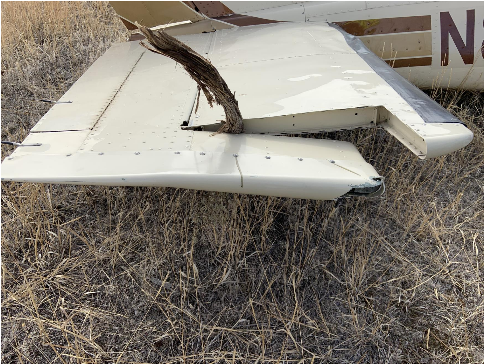
Photo 4 – Accident site, right horizontal stabilizer and elevator. (Courtesy of the Lemhi County Sheriff's Office)
