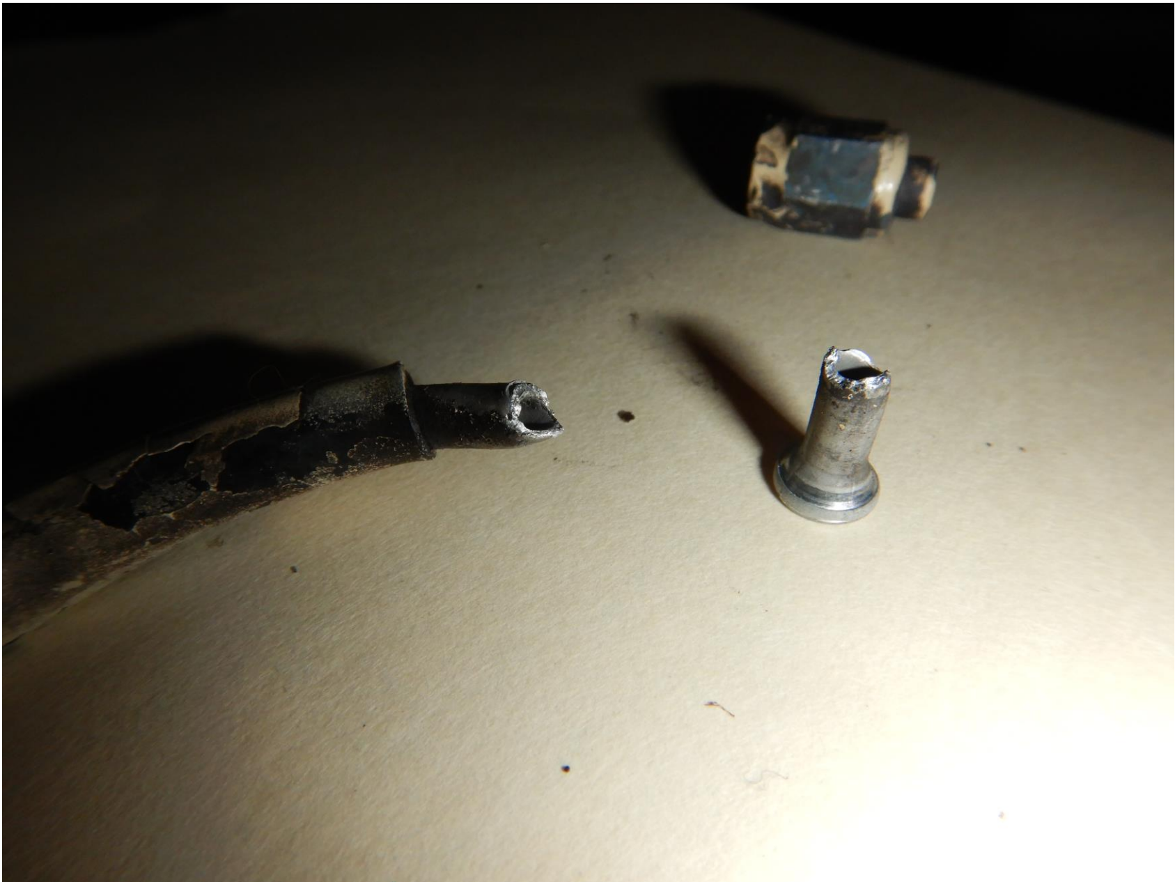
Photo 2 - Right main landing gear brake line separation.
