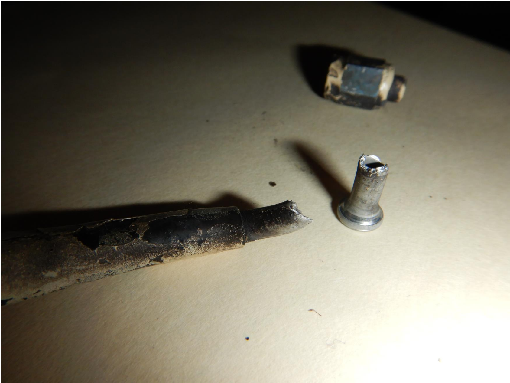
Photo 3 - Right main landing gear brake line separation.
