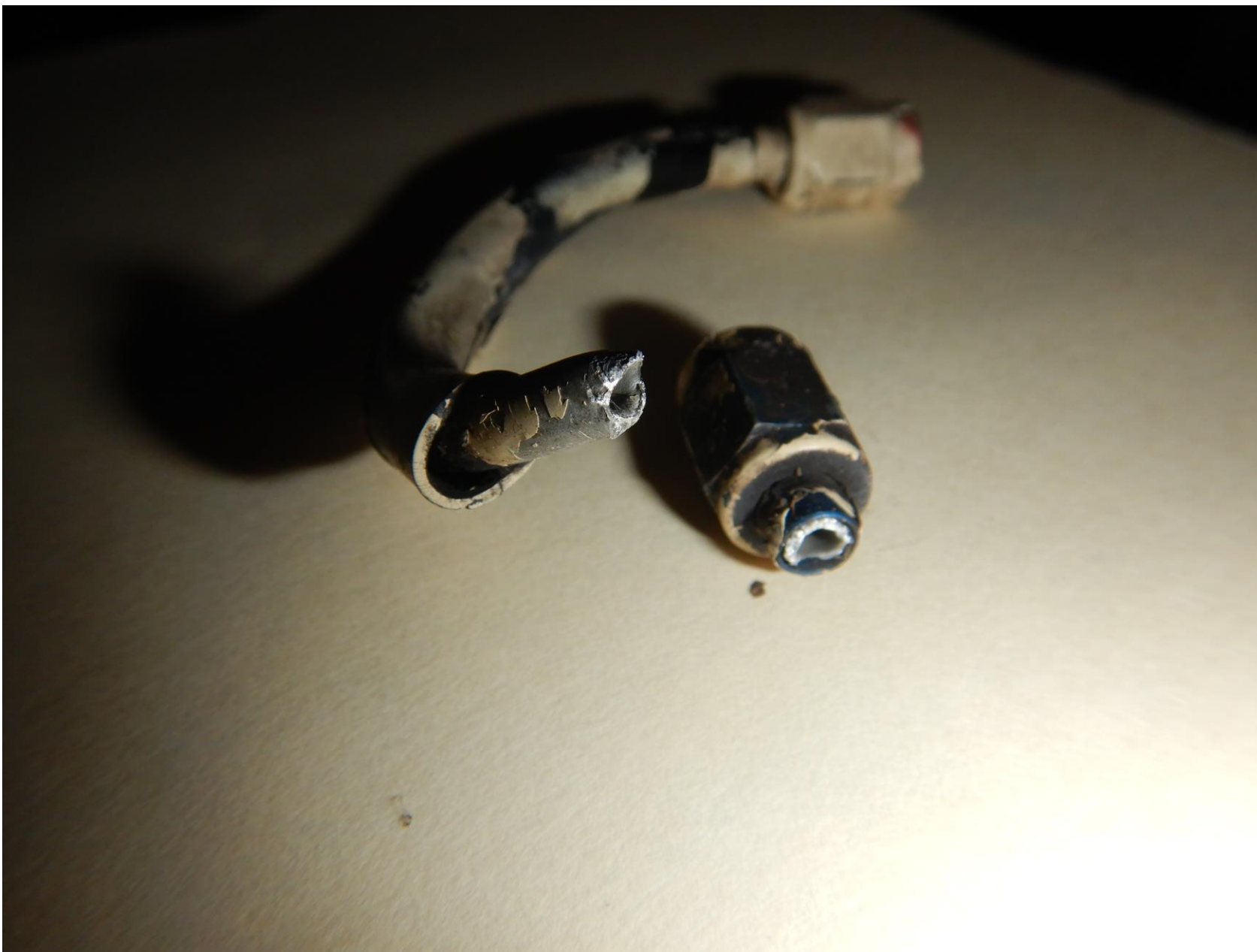
Photo 1 – Right main landing gear brake line separation.
