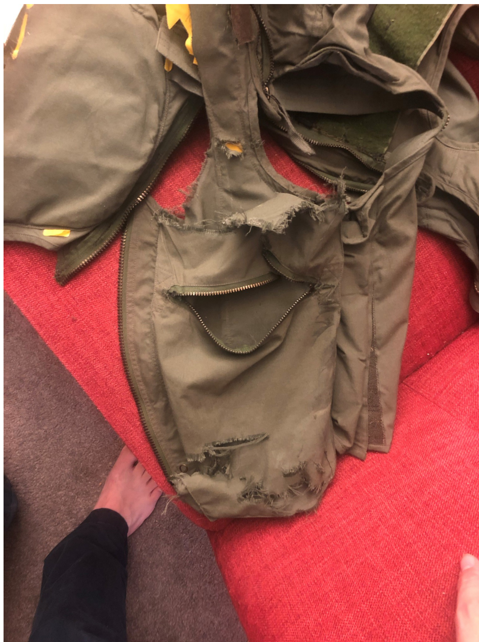
Photo 7 - View of pilot's left leg G-suit damage (photo courtesy of the pilot)
