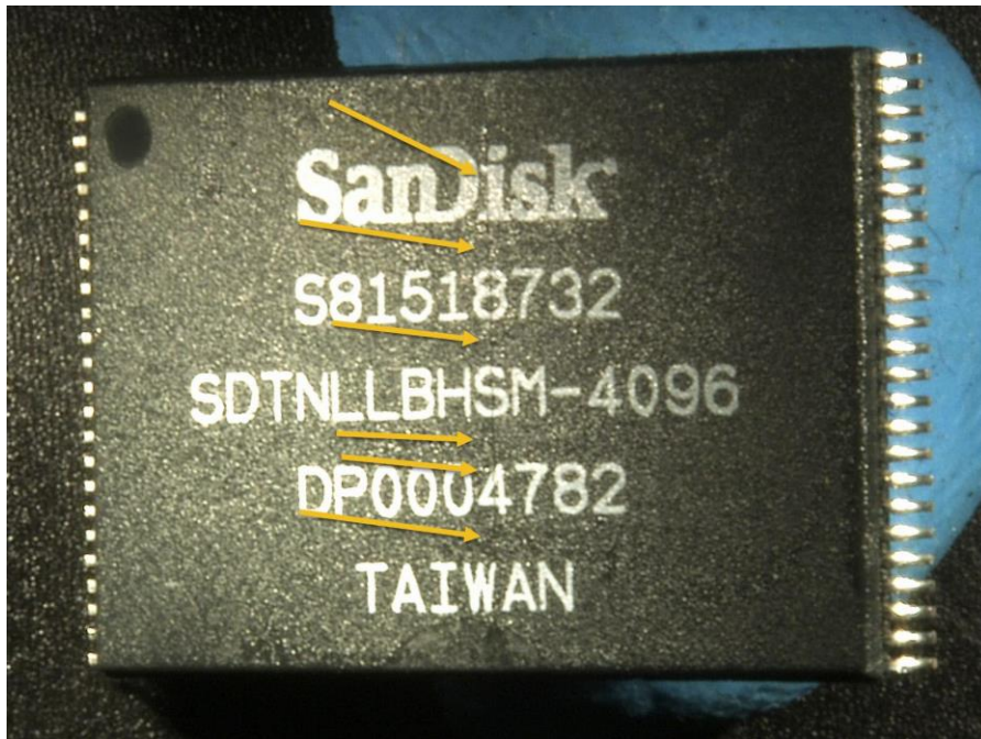
Figure 3. Stereoscopic microscopy photo of 48-pin memory component exhibiting a crack. The crack is annotated.
