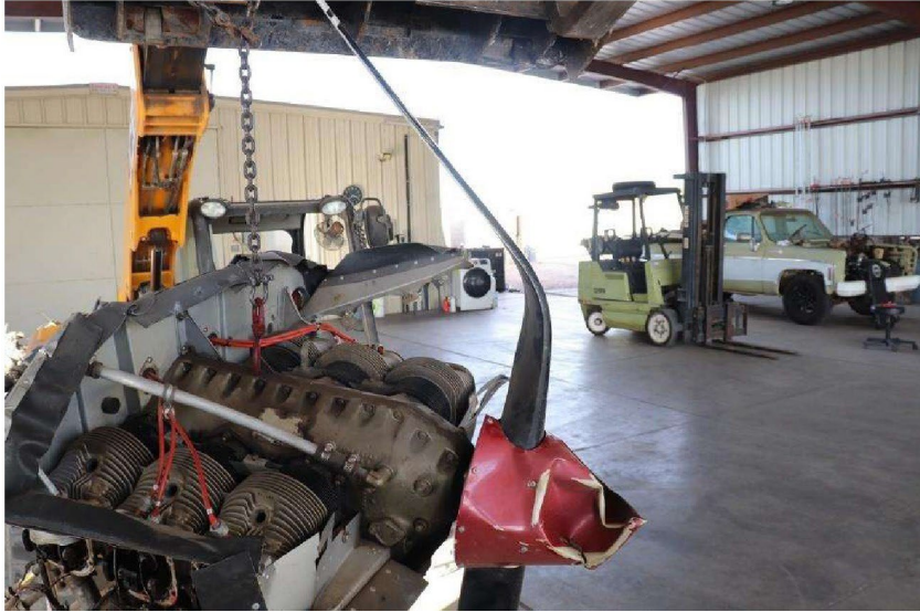
Figure 14-Propellor with bend, courtesy NTSB
