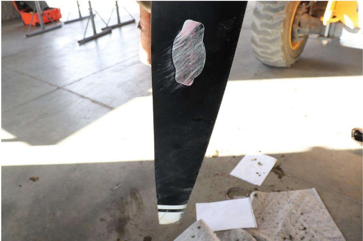
Figure 13-Propel/or Scratches, courtesy NTSB
