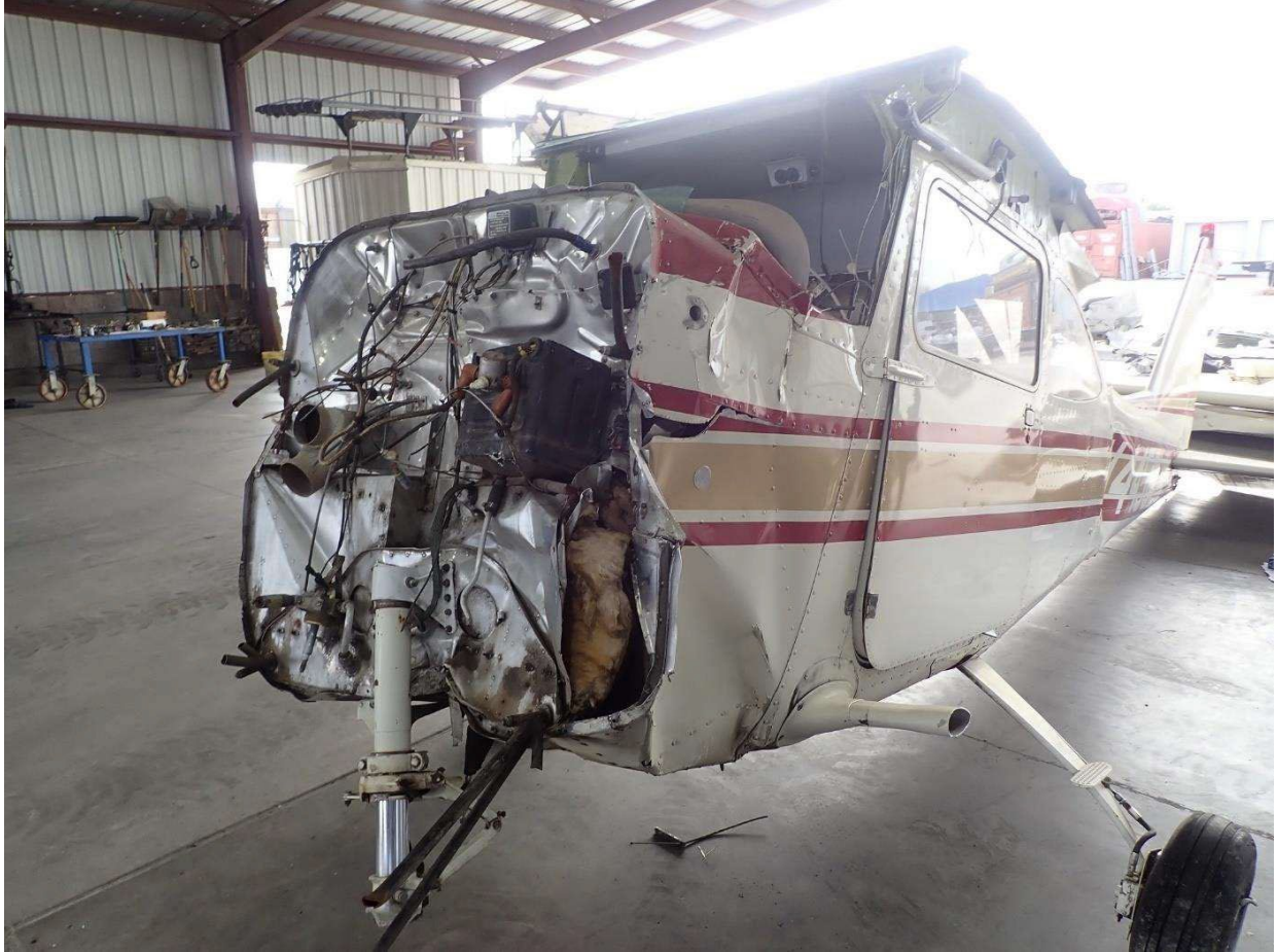
Figure 12-Damage to engine compartment and front wheel, courtesy Textron
