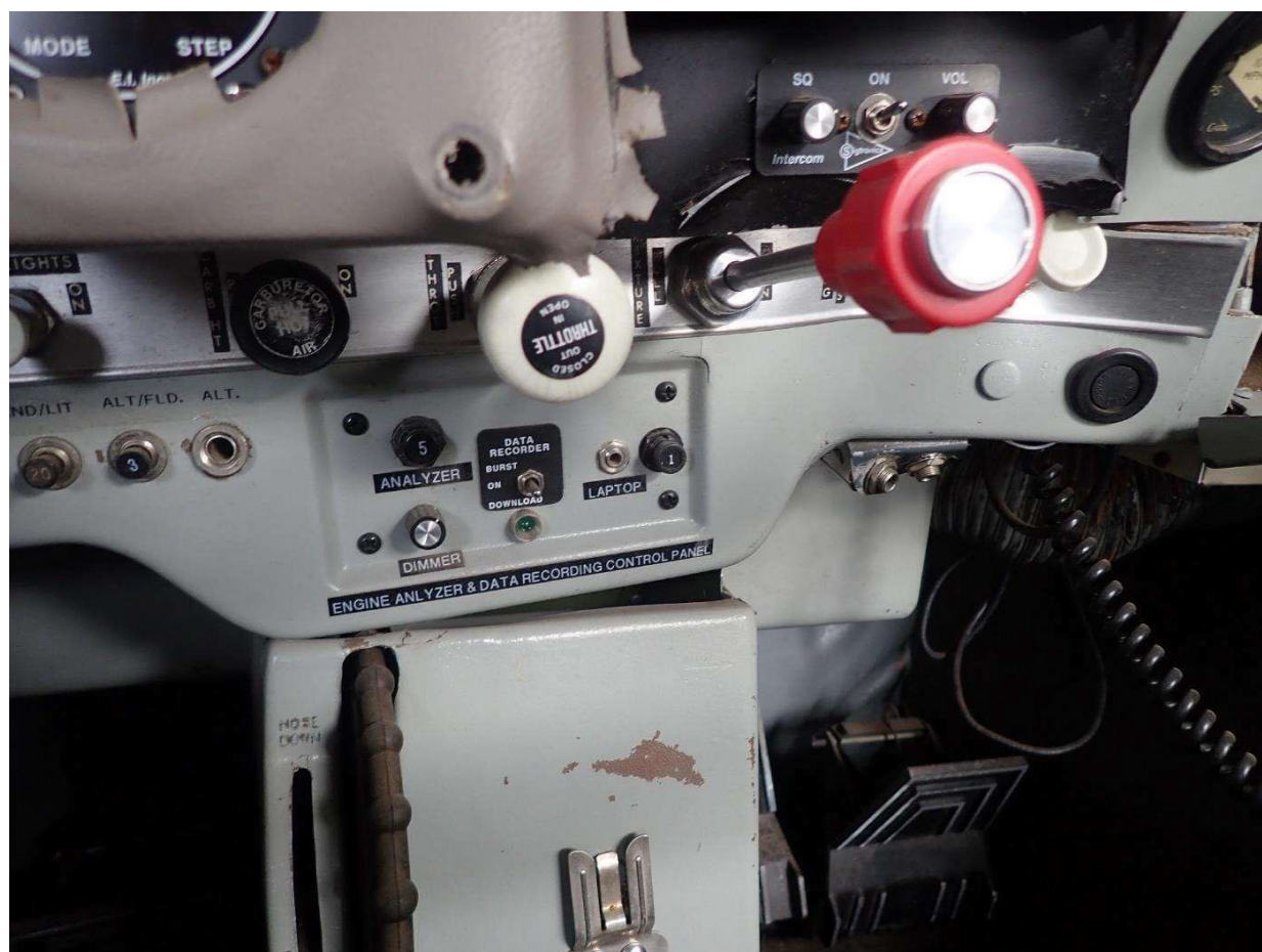
Figure 10-Throttle, mixture, and carburetor heat controls, courtesy Textron
