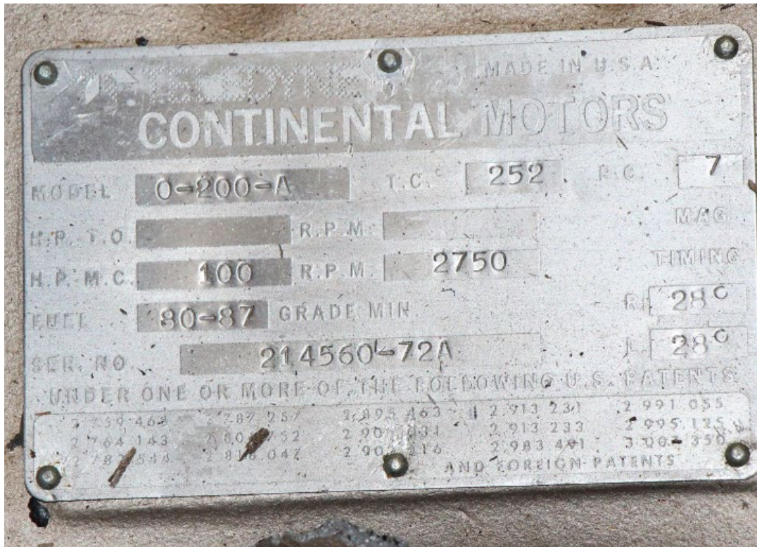
Photograph 1: Engine Data Plate
