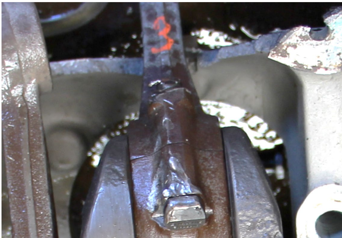
Photograph 8: Cylinder 3 connecting rod with missing castellated nut
