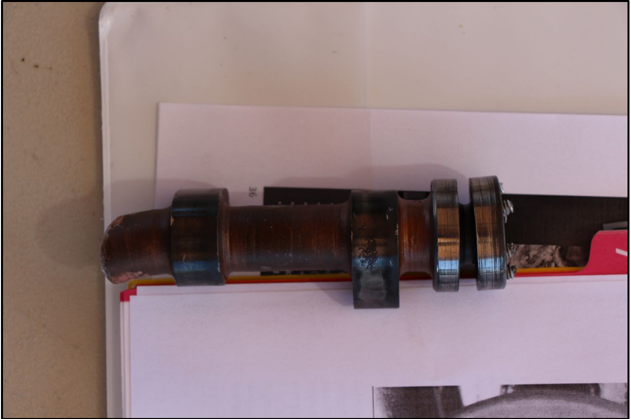
Photograph 5: Fractured Camshaft Section
