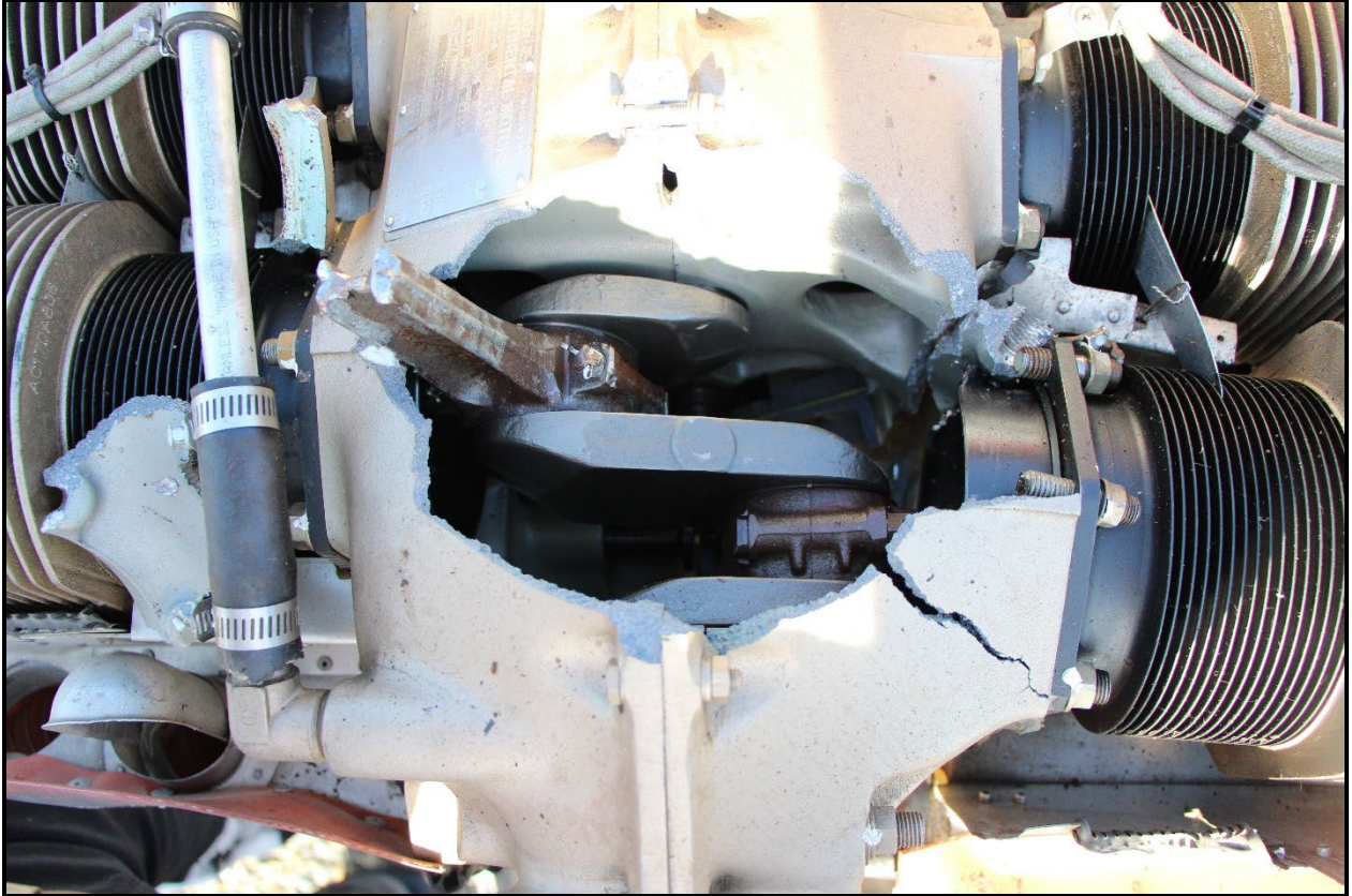
Photograph 3: Hole in Crankcase at Cylinder 3/4 and Exposed Cylinder 3 Connecting Rod Shank
