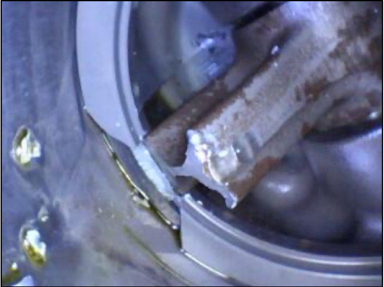
Photograph 4: Cylinder 3 Piston Ring Seal and Piston Ring
