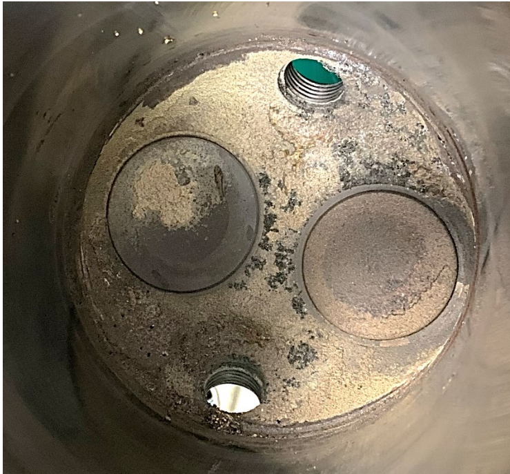
Figure 9. Photograph of the #3 cylinder inner surface showing heavy combustion deposits in the general between the spark plugs, intake and exhaust valves.
