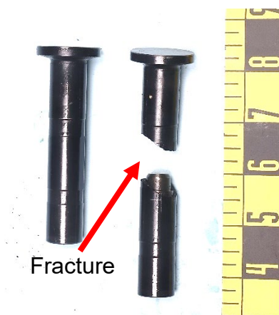
Figure 4. As-received tappets for the #3 cylinder. One of the tappets fractured at the shank portion.
