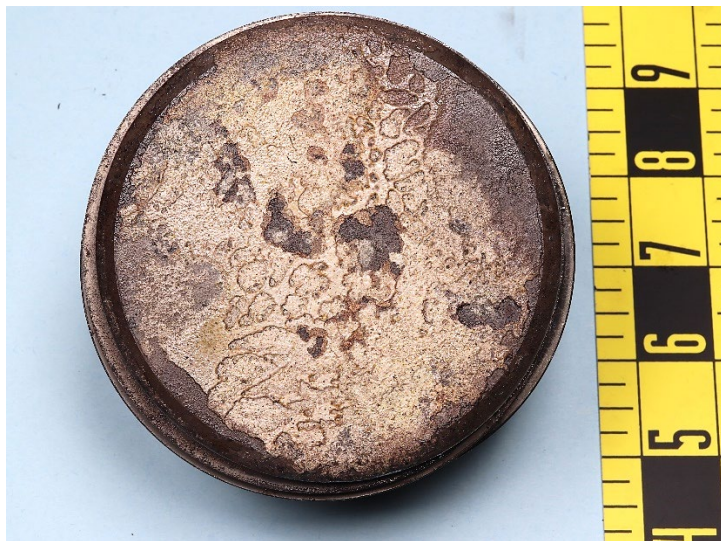
Figure 8. Photograph of the #3 piston showing heavy combustion deposits on the outer surface of the crown portion.
