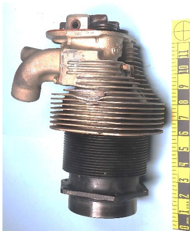
Figure 3. As-received #3 cylinder. Push rods are in the background and are not visible.
